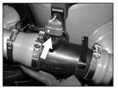
39. Reconnect the mass air sensor electrical connection as shown.
