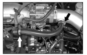
38. Install the provided vent hose onto the cam cover and the intake tube and secure with the provided hose clamps as shown.
