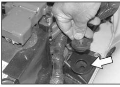
25. Remove the stock rubber grommet from the air cleaner support bracket as shown.
