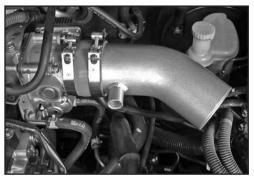
23. Install the throttle body tube onto the throttle body as shown, but do not tighten at this point.
