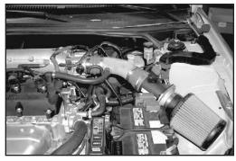
42. This intake kit has been designed to be used in two different configurations. In the case of inclement weather, the cold air tube can be removed and the air filter can be clamped onto the intake tube located in the engine compartment to avoid the possibility of ingesting water into the engine. NOTE: If you have any concerns, return the vehicle to stock using the factory equipment.
