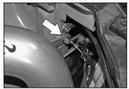
33. Using the bolt removed in step 31, secure the cold air tube bracket and ground wire to the inner fender as shown.
