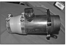
24. Install the silicone hose and hose clamps onto the mass air sensor as shown.
