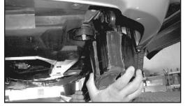
35. From underneath the vehicle install the K&N® air filter onto the cold air tube and secure with the provided hose clamp.
