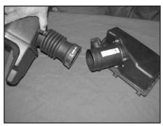
18. Loosen the hose clamp, then, remove the rubber bellows from the mass air sensor as shown.
