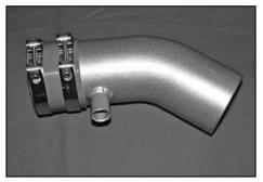
22. Install the silicone hose and hose clamps onto the throttle body tube and tighten as shown.
