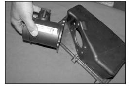
19. Loosen and remove the four bolts that secure the mass air sensor, then, remove the mass air sensor as shown.
