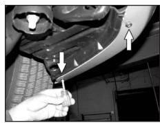
14. From underneath the vehicle loosen and remove the two screws on the lower valance as shown. **NOTE:** It will be necessary to raise the vehicle and secure it with jack stands for this step.
