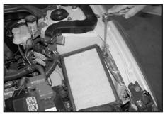
10. Loosen and remove the bolt that secures the lower air cleaner assembly as shown.
