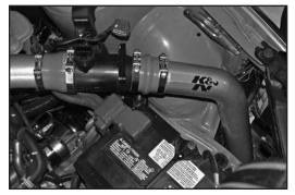
32. Slide the hump hose onto the mass air sensor assembly as shown but do not tighten completely.
