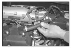
4. Disconnect and remove the crank case vent hose as shown.
