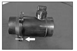
20. Assemble the mass air adapter and the mass air sensor using the provided hardware as shown. NOTE: One of the button head screws is longer than the others and should be placed in the orientation as shown.
