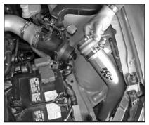
31. Slide the cold air tube into the hole in the inner fender as shown.
