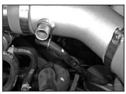
36. Slide the transmission vent hose into the provided wire hanger as shown, then slide the wire hanger onto the vent tube on the throttle body tube as shown
