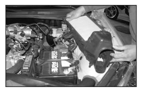
11. Pull firmly upwards to release and remove the lower air cleaner assembly as shown. NOTE: K&N Engineering, Inc., recommends that customers do not discard factory air intake.
