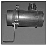
21. Install the bracket onto the mass air sensor using the provided hardware as shown.
