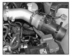
27. Slide the mass air assembly onto the throttle body tube as shown.
