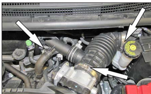
4. Release the spring clamp securing the crank case vent hose to the intake hose and disconnect the hose from the intake tube. Loosen the hose clamps securing the intake hose to the air box and throttle body.
