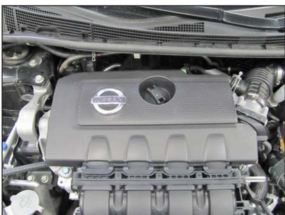
2. Lift up and remove the engine cover.
