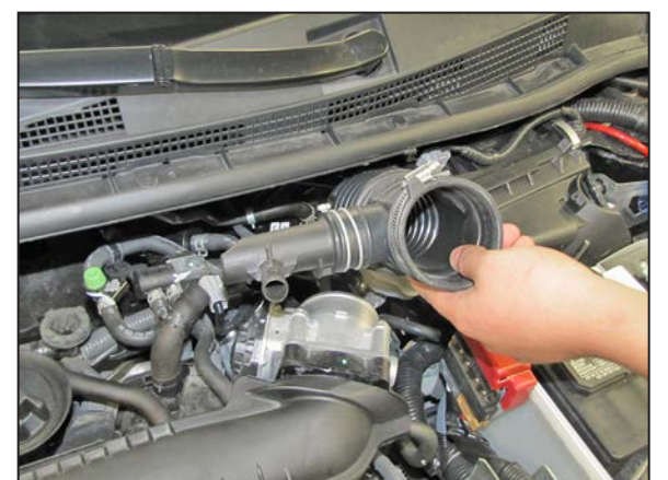
5. Remove the intake hose from the vehicle.
