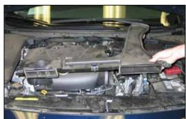
3. Remove the fresh air intake duct from the vehicle as shown.
