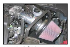
26. Install the K&N® air filter assembly onto the intake tube and secure with the provided hose clamp.
