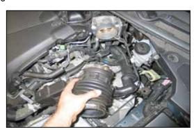
9. Remove the Stock Intake tube and intake tube resonator chambers as shown.
