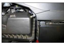
Remove the air box retaining bolt shown.
