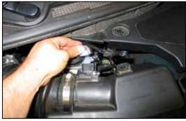
5. Disconnect the mass air sensor electrical connection.
