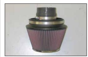
25. Install the  $K\&N^{\otimes}$  air filter onto the air filter adapter assembly as shown.
