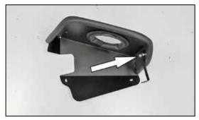
13. Install the mounting bracket (070952) onto the inside of the heat shield using the provided spacer as shown.
