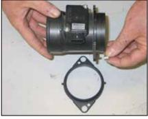
13. Remove the factory gasket and the two spacers from the mass air sensor.
