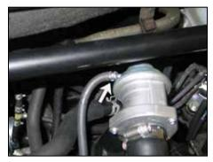
5. Release the spring clamp that secures the bypass valve signal line and then disconnect the bypass valve signal line from the bypass valve.
