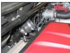
31. Install the silicone hose (08486) onto the turbo outlet and secure with the provided hose clamp.
