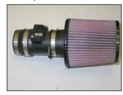
25. Install the K&N® filter onto the mass air sensor and secure with the provided hose clamp.
