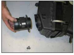
12. Remove the two bolts which secure the mass air sensor to the air box and then remove the mass air sensor from the air box.
