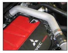
33. Install the K&N® upper intercooler tube into the silicone hose on the turbo outlet, align with the intercooler inlet, slide the silicone hose onto the inlet and then secure with the provided hose clamps.
