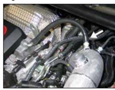
23. Connect the provided crank case vent hose to the remaining ½ NPT fitting and then to the valve cover port as shown.
