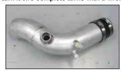
17. Install the silicone hose (084036) onto the K&N® intake tube as shown and secure with the provided hose clamp.
