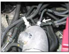
22. Connect the factory vacuum line to the ¼ NPT fitting as shown.
