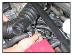
8. Loosen the hose clamps which secure the intake tube to the turbo inlet and mass air sensor. Remove the intake tube partially out of the vehicle and then disconnect the remaining vacuum line. Once the vacuum line is disconnected the complete intake hose assembly can be removed from the vehicle.
