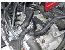
15. Install the tube mounting bracket (070125) onto the transmission/engine lifting bracket location using the factory bolt removed in step #11.
