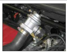
28. Install the cut section of silicone hose (084071) onto the bypass valve and secure with the provided hose clamp.
