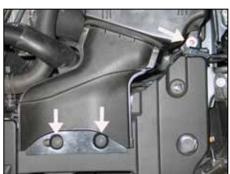
9. Remove the two plastic retaining screws and air box retaining bolt which secure the fresh air scoop as shown.
