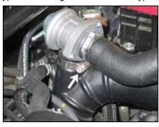
6. Loosen the hose clamp securing the bypass valve to the intake tube and then disconnect the bypass valve from the intake tube, set it to the side.
