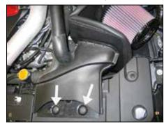
34. Install the fresh air intake scoop into the heat shield as shown and then secure with the factory retaining clips.
