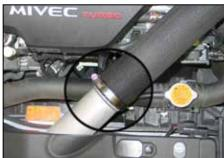
3. Loosen the hose clamps, which secure the upper intercooler hose to the turbo outlet and intercooler inlet.
