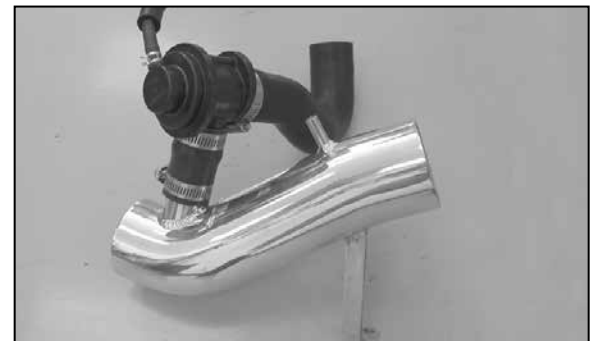
25. Secure the bypass valve to the K&N® intake tube using the provided silicone hose and hose clamps as shown.
