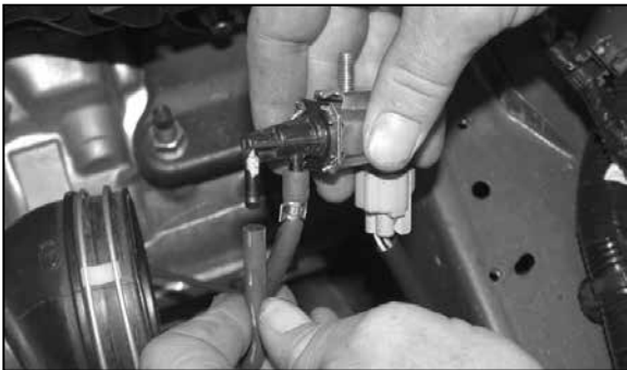
13. Disconnect the vent hose on the solenoid valve as shown.
