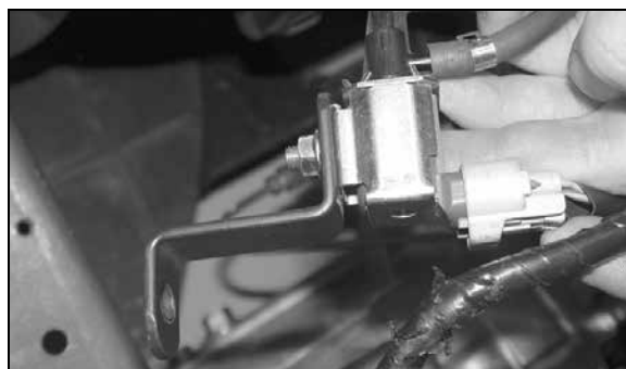
21. Using the hex nut from step 10 secure the solenoid valve to the provided "Z" bracket as shown.
