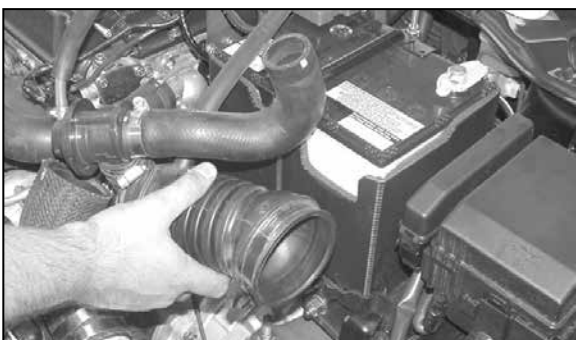
15. Loosen the hose clamp at the turbo inlet and remove the intake tube assembly as shown.
