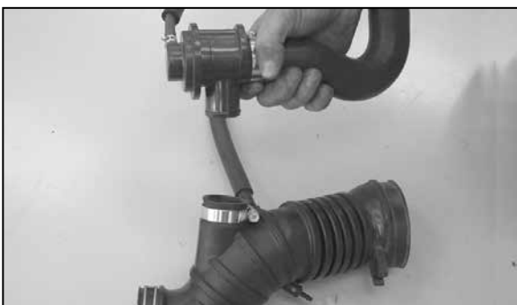
16. Loosen the hose clamp and remove the bypass valve from the intake tube as shown.
