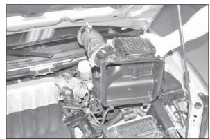
7. Remove the upper air box and intake tube from the vehicle.
