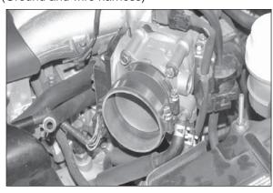
21. Install the provided silicone hose and hose clamps onto the throttle body as shown.
