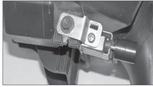
17. Loosen and remove the bolt that secures the fresh air intake door switching valve solenoid to the lower air box.
