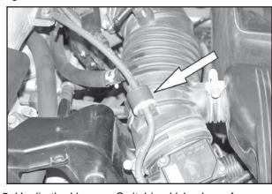
5. Unclip the Vacuum Switching Valve hose from the stock intake tube.
