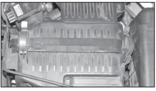
4. Unclip the two clips that hold the air box together.
