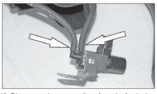
18. Disconnect the vacuum lines from the fresh air door vacuum switching valve.
