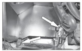
28. Attach the front bracket to the threaded hole on the stock air box mounting point. Attach the fresh air intake door switching valve solenoid and the rear bracket to the other threaded hole with the provided hardware.
