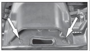
9. Loosen and remove the 2 screws that hold the air inlet duct in place.
