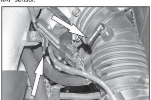
3. Disconnect the crank case vent (CCV) hose and fresh air intake door vacuum switching valve hose, then loosen the hose clamps at the throttle body.
