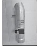
16. Remove the two screws securing the MAF sensor to the factory air box. Install the MAF sensor into the K&N® intake tube with the provided hardware.
