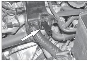
22. Install the "L" Bracket onto the wire harness bracket with the provided hardware.
