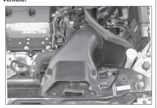
29. Install the factory air inlet duct, and secure with the two screws removed during step # 9. Adjust for fit and clearance, then tighten the heat shield mounting hardware.
