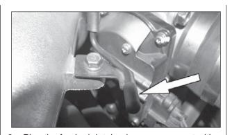
3a. Plug the fresh air intake door vacuum port with the provided rubber cap.
