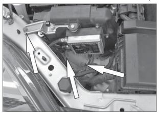
10. Loosen the three bolts that secure the ECU in place.
