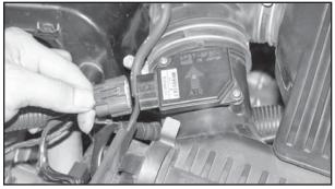
2. Disconnect the MAF sensor harness from the MAF sensor.
