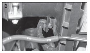
6. Lift the upper air box and turn over (A), then unclip the MAF sensor wire harness (B).
