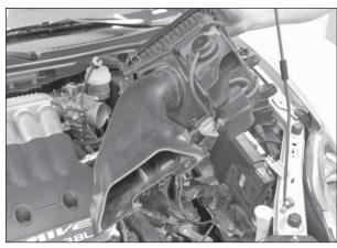
13. Lift the lower air box, pulling up to the left to unclip it.
