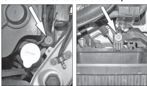
11. Loosen and remove the two bolts that secure the lower air box.
