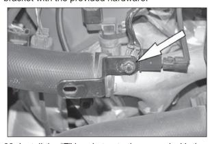
23. Install the "Z" bracket onto the ground with the provided hardware.
