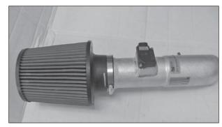
31. Install the K&N® air filter onto the intake tube as shown.
