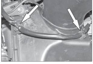
14. Turn the lower air box sideways, then unclip the two clips that secure the wire harness. Remove the lower air box from the vehicle.
