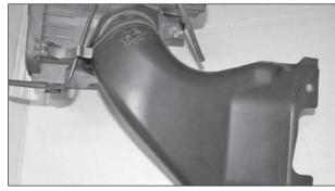
19. Unclip and remove the air inlet duct from the lower air box.
