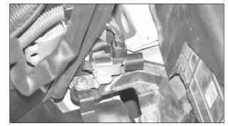
30. Reconnect the fresh air intake door vacuum switching valve solenoid electrical connection.
