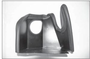
24. Install the small edge trim into the hole, then attach the large edge trim around the heat shield.
