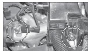
20. Loosen and remove the two specified bolts. (Ground and wire harness)
