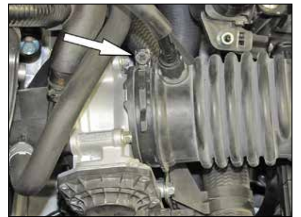
5. Loosen the hose clamp securing the factory intake hose to the throttle body.
