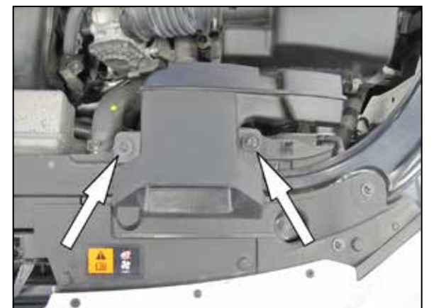
6. Remove the two bolts securing the fresh air intake scoop to the core support.
