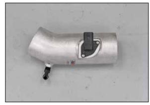
18. Install the mass air sensor into the K&N $^{\odot}$  intake tube and secure with the provided hardware.
