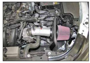
19. Install the K&N<sup>®</sup> Air filter through the heat shield, install the intake tube into the air filter and then into the coupling hose. Adjust the tube and filter for best fit and then secure with the provided hose clamps.
