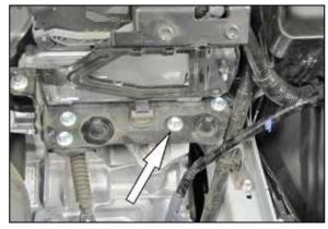
13. Remove the ECU mounting bracket bolt shown. **NOTE: This bolt will be reused in the next step.**
