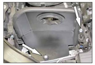
14. Install the heat shield assembly so that the mounting grommet is on the air box mounting stud and the bracket aligns with the bolt hole from the previous step, secure the heat shield using the factory bolt from the previous step.
