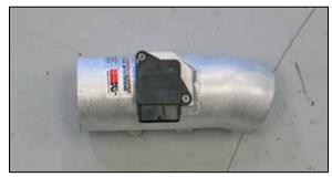
16. Install the mass air sensor into the K&N  $^{\!0}$  intake tube and secure with the provided hardware.
