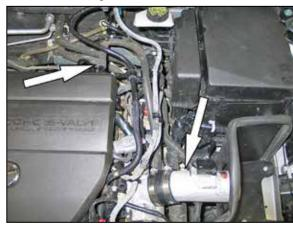
21. Connect the long end of the crank case vent hose to the fitting installed into the K&N® intake tube and then attach the open end to the valve cover port.
