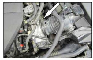
6. Loosen the hose clamp securing the factory intake tube to the throttle body.
