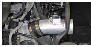
19. Install the K&N® intake tube assembly into the hose at the throttle body and align with the mounting bracket. Secure the tube with the hardware and hose clamp provided.
