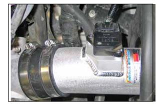
23. Reconnect the mass air sensor electrical connection.
