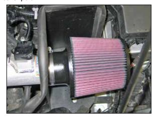
22. Install the K&N® air filter onto the K&N® intake tube and secure with the provided hose clamp. NOTE: Drycharger® air filter wrap; part # RX-4990DK is available to purchase separately.
