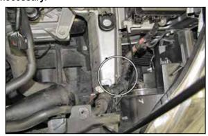
11.Remove the factory body bolt shown from the inner fender.
