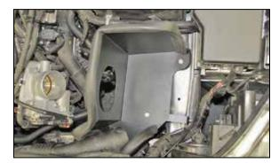
12. Install the heat shield assembly and secure with the provided hardware.
