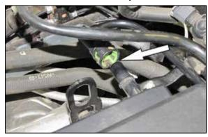
4. Release the green clip and then disconnect the crank case vent hose from the valve cover port.
