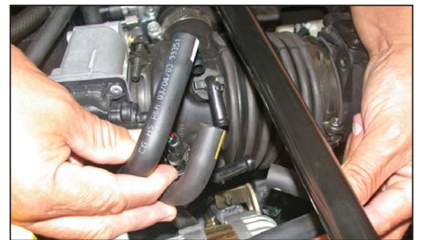
7. Disconnect the three hoses from the stock intake tube as shown. NOTE: On some models there is only 2 vacuum lines.
