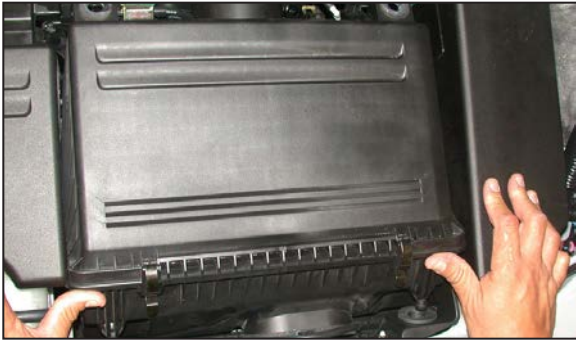
10. Push back on the front of the air cleaner to release the air cleaner from the stock grommets.
