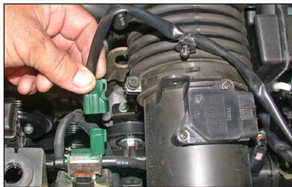
4. On manual transmission vehicle, (automatic transmission vehicles, go to step 7.) disconnect the vacuum switch electrical connection and unclip the wire from the mass air sensor housing as shown. NOTE: Some EU and UK SP-vehicles may have this connection, even if they don't have the vacuum switch!
