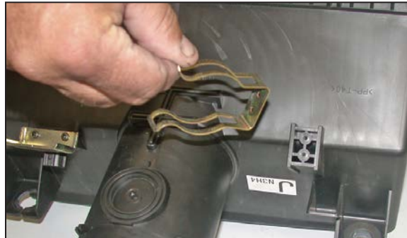
19. On manual transmission vehicles (automatic transmission vehicles go to step 20) remove the vacuum canister clip from the air cleaner assembly.
