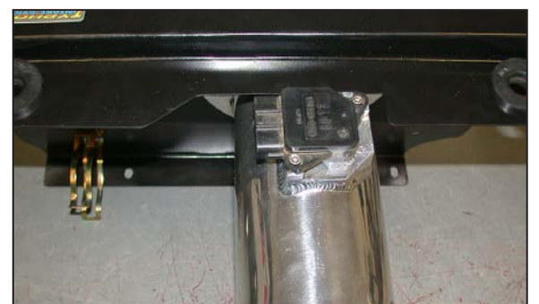
26. Install the mass air sensor into the intake tube using the provided hardware as shown.
