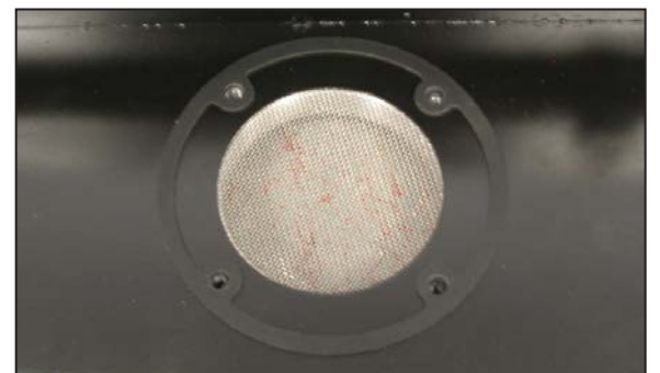
24. Install the heat shield and the remaining gasket onto the filter adaptor as shown.
