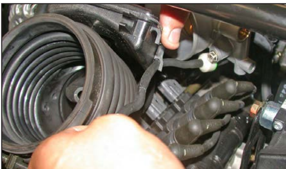
14. Loosen the hose clamp and pull the intake tube off of the throttle body, rotate the tube and unclip the vacuum hose from the intake tube as shown.
