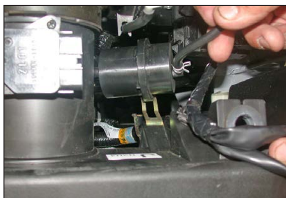
6. On manual transmission vehicles, remove the vacuum hose from the resonator as shown.
