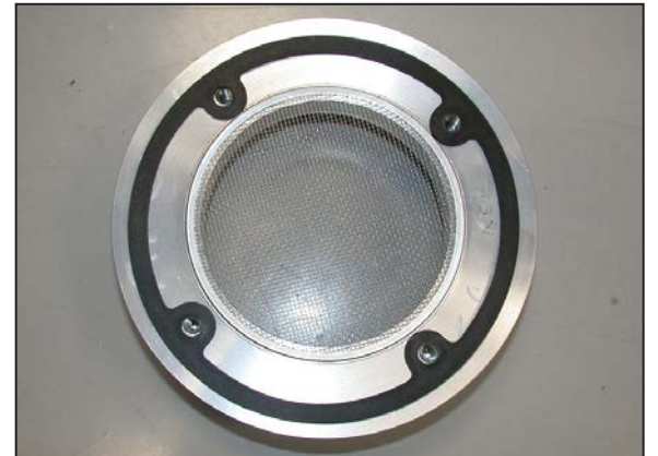
23. Install the stock screen and the provided gasket onto the back of the provided filter adapter as shown.
