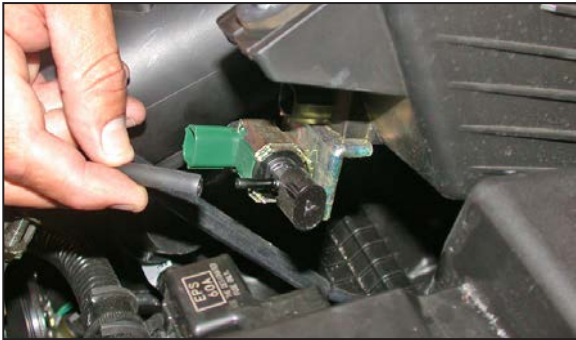
11. Lift the air cleaner upwards, then disconnect the vacuum hose from the vacuum switch (automatic transmission vehicles disregard the vacuum switch hose and go to step 12.) as shown.
