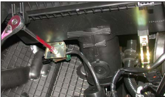
13. On manual transmission vehicles (automatic transmission vehicles go to step 14) turn the air cleaner upside down to remove the nut that secures the vacuum switch to the air cleaner assembly then remove the vacuum switch.
