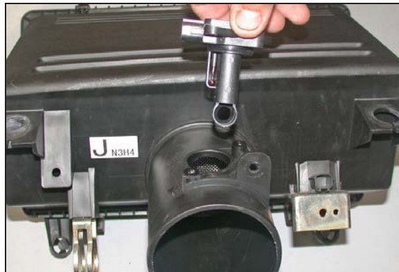
17. Remove the mass air sensor from the air cleaner housing as shown.
