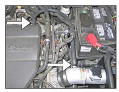
21. Install the provided crankcase vent hose onto the fitting installed into the K&N® intake tube. Attach the other end of the crankcase vent hose to the valve cover port.
