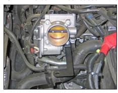
13. Install the bolt removed in the previous step through the tube mounting bracket (083137). Install the bracket onto the throttle body as shown. **NOTE: Do not completely tighten at this time.**
