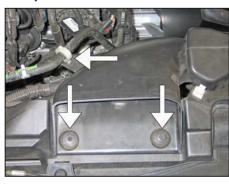
23. Feed the fresh air scoop's outlet into the heat shield while also attaching the inlet back onto the core support. Secure the scoop with the factory bolts that were removed in step #4 and attach the coolant hose with the factory clip.
