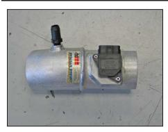
10. Install the 5/8"NPT fitting into the K&N® intake tube as shown.
