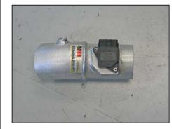
9. Install the mass air sensor into the K&N® intake tube and secure with the provided hardware.
