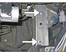
18. Set the two provided  $\frac{1}{2}$ " spacers onto the inner fender over the airbox mounting bracket bolt holes.
