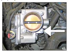
12. Remove the rear lower throttle body mounting bolt shown.
