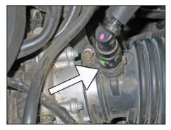
4. Loosen the hose clamp that secures the stock intake tube to the throttle body.
