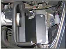
19. Set the heat shield assembly into position on the inner fender and then secure to the inner fender with the provided hardware.
