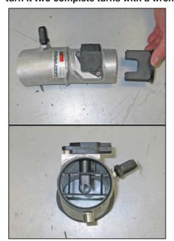
11. Apply a thin coat of the provided super glue to the lip of the air straightener and then install the straightener into the intake tube as shown.
