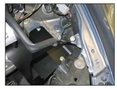
20. Secure the heat shield mounting bracket to the core support with the provided spacer and hardware.
