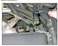
3. Release the green locking clip, then disconnect the crankcase vent line from the valve cover.
