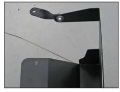
16. Install the heat shield mounting bracket (07105) onto the heat shield using the provided hardware.
