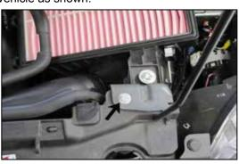
6. Remove the lower airbox mounting bolt shown.
