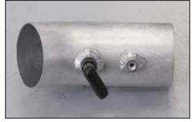
16. Install the 90° vent fitting into the K&N® intake tube as shown.
