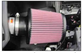
23. Install the K&N<sup>®</sup> air filter onto the K&N<sup>®</sup> intake tube and secure with the provided hose clamp.
