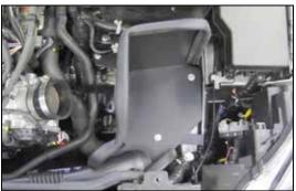
15. Set the heat shield into position on the rubber mounted stud, and then secure the heat shield with the provided hardware.
