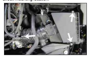
3. Release the two upper airbox retaining clips and loosen the hose clamp which secures the intake tube to the throttle body.
