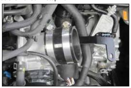
11.Install the provided silicone hose (08756) onto the throttle body and secure with the provided hose clamp.
