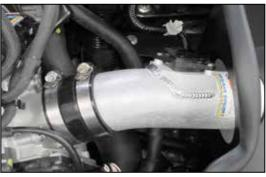
20. Install the K&N<sup>®</sup> intake tube assembly into the silicone hose at the throttle body and align with the tube mounting bracket and then secure with the provided hardware and hose clamps.
