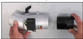
19. Insert the venturi insert into the K&N® intake tube as shown.
