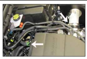
22. Install the short length of the crankcase vent hose onto the valve cover port and then attach the open end to the fitting installed into the K&N® intake tube.
