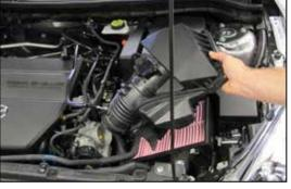
5. Remove the upper airbox assembly from the vehicle as shown.
