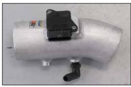
18. Install the mass air sensor into the K&N<sup>®</sup> intake tube and secure with the provided hardware.
