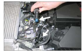
4. Release the blue locking tabs on the crank case vent hose where it attaches to the stock intake tube and then unhook the crank case vent hose from intake tube.
