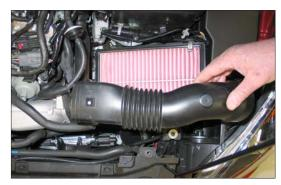
10. Unhook the fresh air duct from the air box and then remove it from the vehicle.
