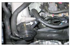
23. Remove the pop off valve upper mounting bolt shown.
