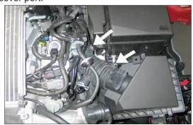
6. Loosen the two hose clamps which secure the intake tube to the air filter and turbo inlet tube.
