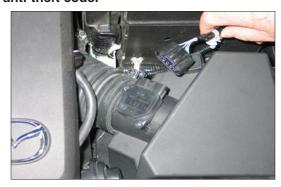
2. Disconnect the mass air sensor electrical connection and unhook the wiring harness from the air box.
