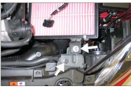
9. Remove the two bolts shown and then remove the front air box mounting bracket from the vehicle. NOTE: The bolt which secures the bracket to the core support will be reused in a later step.
