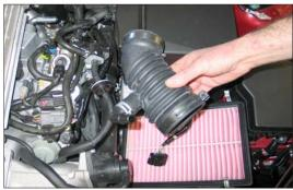
8. Remove the intake tube from the vehicle.
