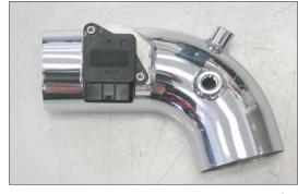
20. Install the mass air sensor into the K&N<sup>®</sup> intake tube and secure with the provided hardware.
