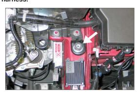
15. Install the provided rubber mounted stud onto the air box mounting bracket as shown using the provided hardware.
