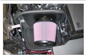
27. Install the K&N® air filter onto the intake tube and secure with the provided hose clamp.
