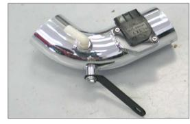
22. Install the tube mounting bracket (083130) onto the  $K\&N^{\circledcirc}$  intake tube as shown.
