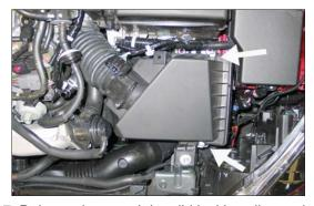
7. Release the two air box lid locking clips and then remove the air box lid from the vehicle.
