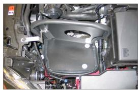
18. Install the heat shield into position on the air box mounting bracket then secure the heat shield with the provided hardware.
