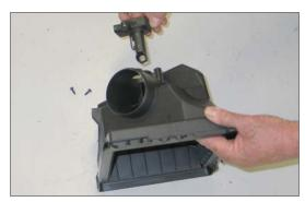
19. Remove the screws securing the mass air sensor and then remove the mass air sensor from the upper air box.
