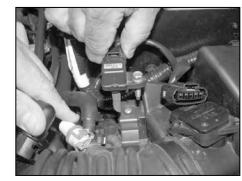
7. Remove the switch/sensor from the air cleaner cover as shown.
