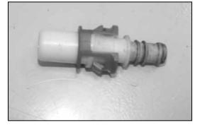
18. On vehicles equipped with the crankcase quick disconnect fitting, slide the plastic clip from step 15 back onto the crankcase vent as shown.
