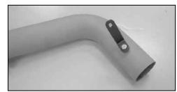
33. Install the provided bracket onto the cold air tube using the provided hardware as shown.
