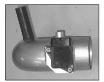
26. Install the mass air sensor into the intake tube using the provided hardware as shown.
