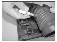
17. On vehicles equipped with the crankcase quick disconnect fitting, remove the plastic vent from the stock intake tube as shown.
