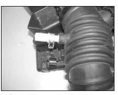
16. On vehicles equipped with the crankcase quick disconnect fitting, slide the hose clamp off rubber crankcase vent flange as shown.
