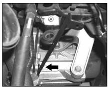
23b. Attach the tube mounting bracket (#06481) to the transmission using the bolt removed in the previous step, as shown.
