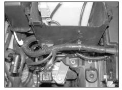
13. Unclip the wire harness from the side of the battery box as shown.
