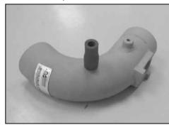
25.On vehicles equipped with the crankcase quick disconnect fitting, install the provided rubber hose onto the vent on the K&N<sup>®</sup> intake tube as shown.
