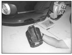
38. Install the air filter onto the cold air tube from underneath the vehicle as shown.
