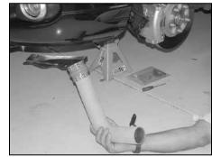
34. From underneath the vehicle install the cold air tube as shown.
