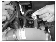
29. On vehicles equipped with the crankcase quick disconnect fitting, install the crankcase vent from step 18 into the silicone hose on the intake tube as shown.
