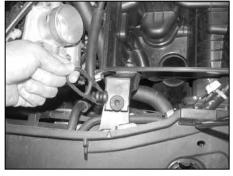
11. Remove the rubber retainer from the core support as shown.
