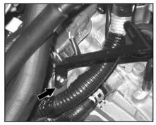
23. On vehicles equipped with an automatic transmission, attach the tube mounting bracket (#06479) onto the transmission control cable bracket using the provided hardware. **NOTE: Do not completely tighten at this time.**
