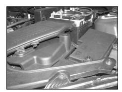
4. Slide the battery cold air vent backwards and remove from the engine compartment as shown.
