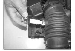
15. On vehicles equipped with the crankcase quick disconnect fitting, remove the plastic clip from the crankcase vent on the stock intake tube as shown. **NOTE: Be careful not to damage as this piece will be reused in a later step.**
