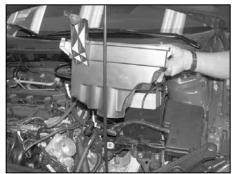
12. Remove the lower air cleaner assembly as shown.
