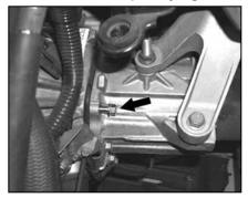
23a. On vehicles equipped with a manual transmission, remove the transmission bellhousing bolt shown.
