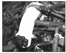
27. Install the K&N<sup>®</sup> intake tube into the silicone hose at the throttle body and align with the mounting bracket. Secure the tube with the provided hardware and hose clamp.
