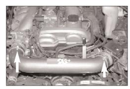
18. Slide the mass air sensor into the silicone hose, then, tighten all hose clamps as shown.
