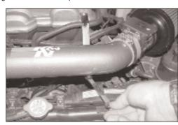
20. Tighten the hex bolt on the  $K\&N^{\otimes}$  intake tube as shown.
