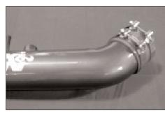
13. Install the silicone straight hose and hose clamps onto the  $K\&N^{\circ}$  intake tube as shown.
