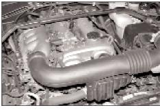
6. Loosen the hose clamps at the throttle body and at the mass
