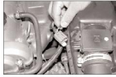
2. Disconnect the mass air sensor electrical connection as
