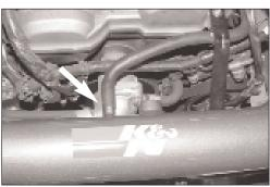
21. Install the crankcase vent hose onto the  $K\&N^{\circledcirc}$  intake tube as shown.
