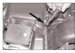
3. Remove the air temperature sensor from the air cleaner assembly as shown.
