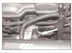
22. Slide the air temperature sensor into the bung on the K&N  $^{\! \otimes}$  intake tube as shown.
