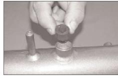
14. Install the silicone sleeve into the air temperature sensor bung on the K&N® intake tube as shown.
