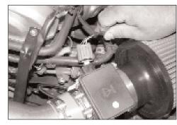
23. Reconnect the mass air sensor electrical connection as shown.
