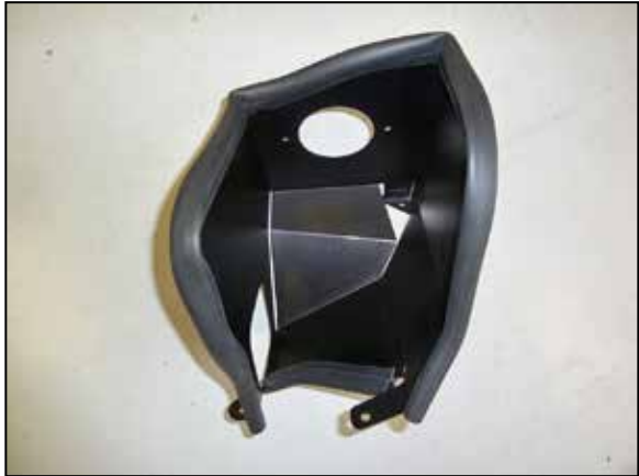
9. Install the 40.5" long edge trim onto the heat shield as shown.
