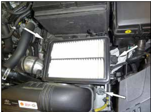
7. Remove the three bolts that secure the lower air filter housing and then remove the housing from the vehicle. NOTE: K&N Engineering, Inc., recommends that customers do not discard factory air intake.
