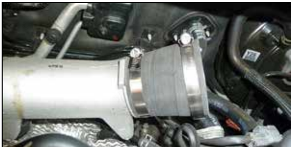
14. Install the provided coupler (08096) onto the turbo inlet and secure with the provided hose clamp.
