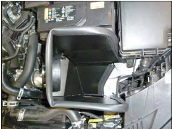
11. Install the heat shield into the vehicle as shown and secure with the provided hardware.
