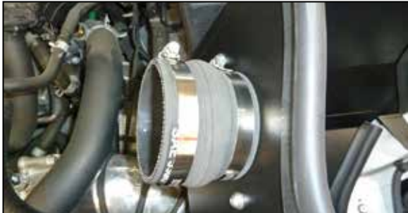
15. Install the provided coupler (087121) onto the filter adapter and secure with the provided hose clamp.
