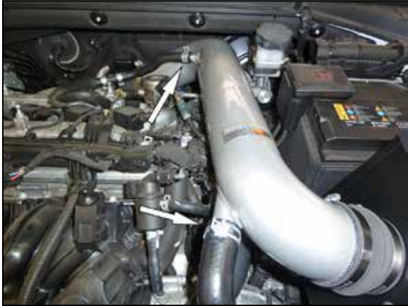
17. Connect the PCV vent and BOV hose to the K&N® intake tube and secure with the factory spring clamps.
