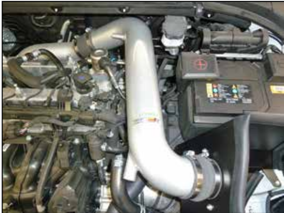
16. Install the K&N® intake tube into the coupler at the turbo inlet and then at the filter adapter, adjust the tube for best fit and then secure with the provided hose clamp.
