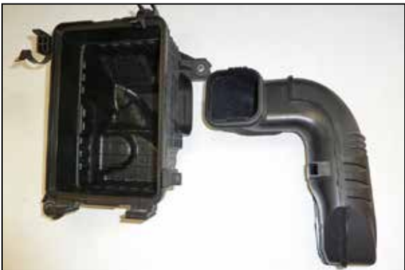
12. Separate the fresh air duct from the factory air filter housing.
