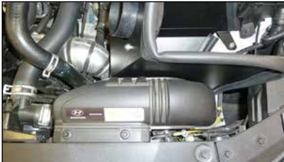
13. Install the fresh air duct into the heat shield and secure it to the original location with the factory retaining pins.
