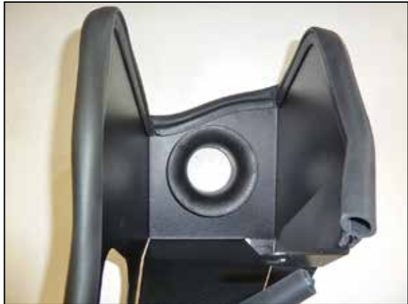
10. Install the filter adapter into the heat shield and secure with the provided hardware.
