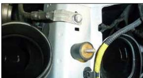
11. Install the provided rubber mounted stud onto the frame rail as shown.
