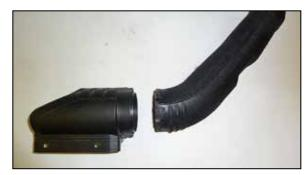
19. Remove the fresh air duct from the scoop. **NOTE:The duct is glued to the scoop.**
