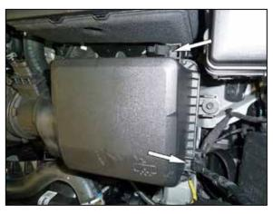
5. Release the two upper air filter housing retaining clips and then remove the upper air filter housing and intake hose from the vehicle.
