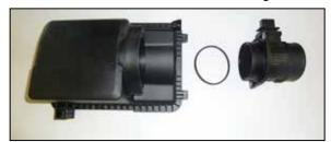
8. Remove the two bolts and then remove the mass air sensor housing from the air filter housing. Remove the O-ring from the mass air sensor housing.
