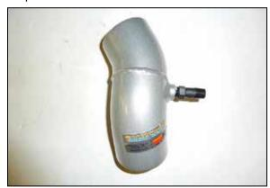
15. Install the provided PCV fitting into the K&N<sup>®</sup> intake tube as shown.
