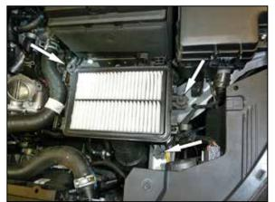
6. Remove the three bolts that secure the lower air filter housing and then remove the lower air filter housing.
