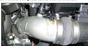
16. Install the intake tube into the couplers and adjust for best fit and then secure with the provided hose clamps.
