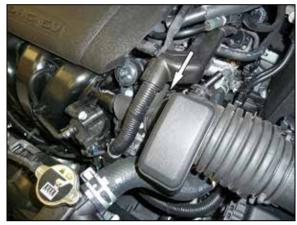
4. Loosen the hose clamp that secures the intake hose to the throttle body.
