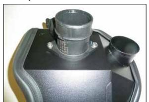
10. Using the provided hardware, secure the mass air sensor into the heat shield as shown.
