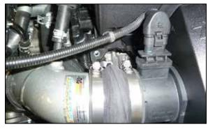
17. Reconnect the mass air sensor electrical connection and connect the factory PCV hose to the fitting installed into the K&N<sup>®</sup> intake tube.
