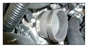
13. Install the provided coupler (08440) onto the throttle body and secure with the provided hose clamp.
