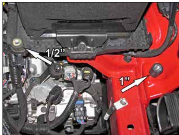
14. Install the provided rubber isolator mounts as shown.
