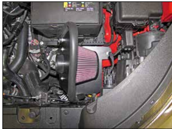
15. Set the heat shield into the engine compartment and secure it to the isolators and core support with the provided hardware. NOTE: Be sure to use a spacer between the bracket and core support. Check to make sure that the hood release cable is secured in its original location.
