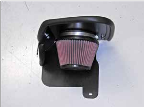
10. Install the K&N® air filter onto the filter adapter and secure with the provided hose clamp. NOTE: Drycharger® air filter wrap; part # RU-5163DK is available to purchase separately.
