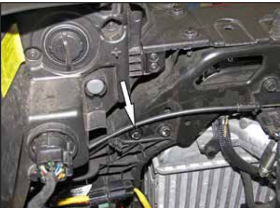
11. Remove the outer most core support bolt shown. NOTE: The hood release cable may be unhooked from its retaining position to ease removal of the bolt.
