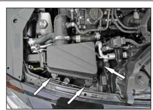
5. Remove the three bolts that secure the driver
