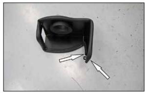
11. Install the edge trim onto the driver side heat shield as shown.
