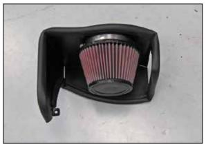
20. Install the remaining air filter onto the passenger side filter adapter as shown and secure with the provided hose clamp.
