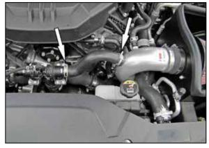
17. Install the passenger side BOV hose onto the driver side intake tube and BOV valve, secure with the factory spring clamps. Connect the vent lines to the fittings installed into the  $K\&N^{\odot}$  intake tube.
