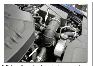
3. Release the spring clamps that secure the two
