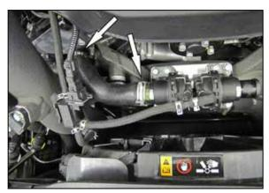
7. Release the spring clamps that secure the passenger side BOV hose to the BOV and intake tube, then remove the driver side BOV hose. **NOTE: This hose will be reused.**
