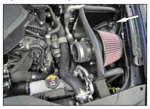
13. Install the driver side heat shield assembly into the vehicle so the fresh air intake inserts into the opening of the heat shield and then secure the heat shield with the provided hardware. Install the coupling hose (084036) onto the filter adapter and secure with the provided hose clamp.
