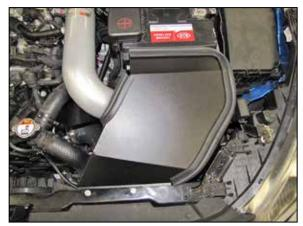
24. Install the heat shield and secure it to the heat shield and core support using the provided hardware.
