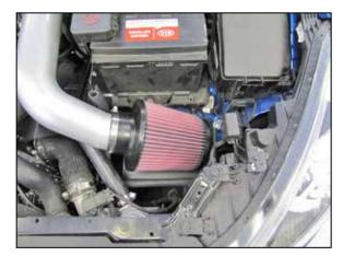
22. Install the  $K\&N^{\otimes}$  air filter and secure with the provided hose clamp.
