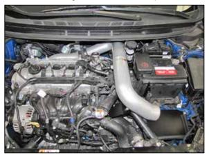
19. Install the K&N® intake tube into the coupler at the turbo inlet tube and align with the mounting bracket previously installed. Secure the tube with the hardware and hose clamp provided.
