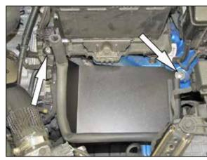
16. Install the heat shield onto the air filter housing mounting locations and secure with the provided hardware.
