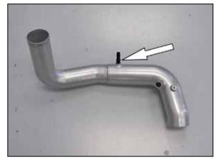
17. Install the provided vent fitting into the K&N® intake tube as shown.
