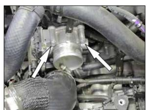
10. Loosen the hose clamp securing the intake charge tube and then remove it from the throttle body. Loosen and remove the two upper throttle body bolts shown.
