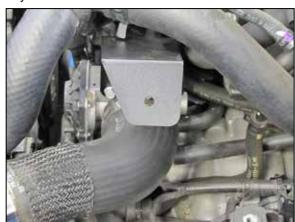
11. Install the provided tube mounting bracket using the factory throttle body bolts removed in the previous step, Reinstall the intake charge hose and secure with the factory hose clamp.
