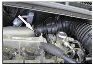
4. Loosen the clamp securing the intake tube to the turbo inlet pipe.
