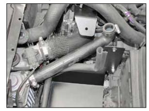
18. Install the provided BOV hose onto the BOV valve but do not tighten the hose clamp at this time.
