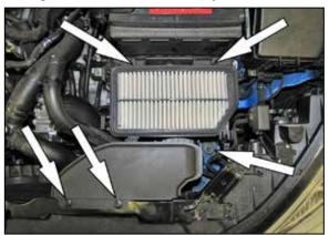
6. Release the two retaining clips securing the fresh air duct and then remove the three bolts securing the lower air filter housing and remove the lower air filter housing assembly.
