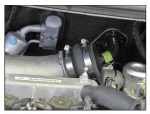
12. Install the provided coupling hose (08185) onto the turbo inlet tube and secure with the provided hose clamp.
