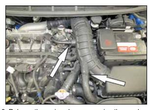
3. Release the spring clamps securing the crank case vent and BOV hose to the intake hose and disconnect the hoses from the intake hose.
