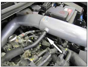
21. Connect the crank case vent hose to the  $K\&N^{\otimes}$  intake tube and secure with the factory hose clamp.
