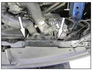
8. Remove the two bolts that secure the inner fresh air duct to the core support and then remove the inner fresh air duct.
