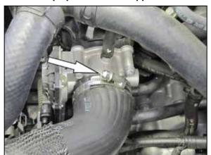
9. Remove the cover from the hose clamp screw on the throttle body charge hose.
