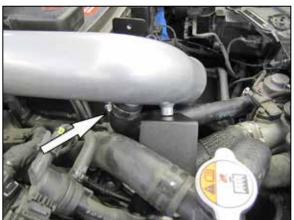
20. Connect the BOV hose to the K&N® intake tube and secure with the provided hose clamp.
