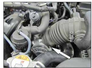
6. Loosen the hose clamp securing the intake tube to the throttle body.
