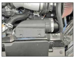
22. Install the fresh air intake scoop and secure it to the heat shield with the provided hose clamp and factory retaining pins.
