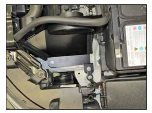
12. Set the heat shield onto the rubber mounted studs install previously and secure with the provided hardware. Tighten all of the hardware securing the heat shield.
