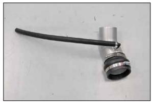
17. Install the provided crank case vent hose onto the fitting installed into the K&N® intake tube as shown and secure with the provided hose clamp.
