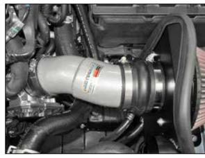
18. Install the K&N® intake tube into the coupling hose at the throttle body, slide the coupling hose onto the filter adapter and then adjust the tube for best fit and secure with the provided hose clamps.
