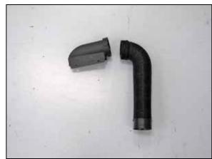
20. Separate the fresh air intake scoop from the duct.
