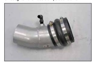
16. Install the  $90^{\circ}$  vent fitting into the K&N<sup>®</sup> intake tube as shown.
