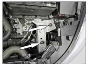
8. Install the two provided rubber mounted studs into the inner fender as shown.
