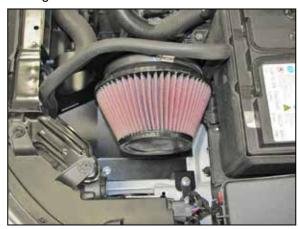
13. Install the K&N® air filter onto the filter adapter and secure with the provided hose clamp.
