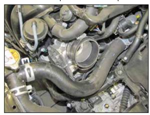
14. Install the provided coupling hose (084036) onto the throttle body and secure with the provided hose clamp.
