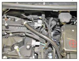
19. Connect the crank case vent hose to the fitting on the valve cover and secure with the provided hose clamp.
