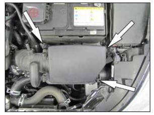
7. Remove the three bolts that secure the air filter housing to the inner fender and then remove the air filter housing and intake tube from the vehicle.
