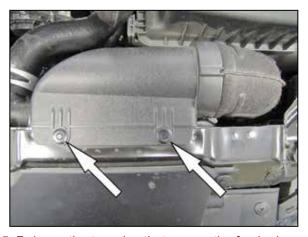
5. Release the two pins that secure the fresh air intake scoop to the core support and then remove the fresh air intake scoop from the vehicle.
