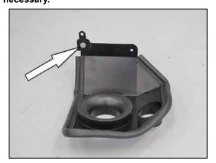
11. Install the provided bracket (07133) onto the heat shield using the provided hardware.
