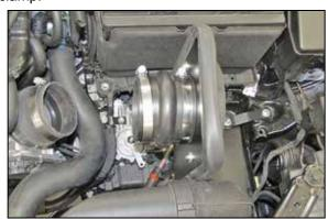
15. Install the hump hose (5-576) onto the filter adapter and secure with the provided hose clamp.
