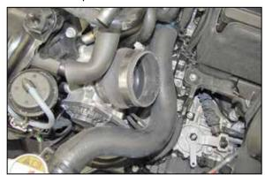
14. Install the provided hump hose (08421) onto the throttle body and secure with the provided hose clamp.
