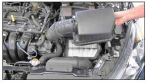
5. Release the two upper air box retaining clips. Separate the upper air box from the lower air box, disconnect the intake hose from the throttle body and then remove the assembly from the engine.
