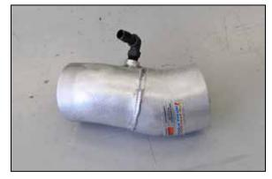
16. Install the 90° vent fitting into the K&N® intake tube as shown.
