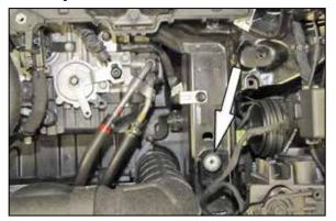
12. Install the 1" tall rubber mounted stud into the forward air box mounting location as shown.
