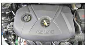
2. Pull up the engine cover to release it from the mounting grommets and then remove the cover from the engine.
