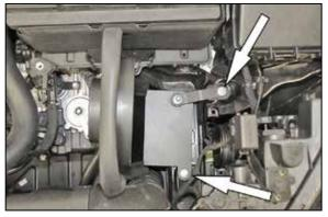
13. Install the heat shield onto the inner fender and secure with the provided hardware as shown.
