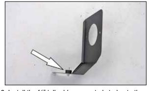
8. Install the  $\frac{1}{2}$ " tall rubber mounted stud onto the heat shield using the provided hardware.
