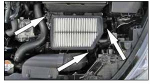
6. Loosen and remove the three bolts securing the lower air box to the inner fender.
