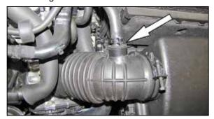
3. Release the spring clamp securing the crank case vent hose to the factory intake hose and then disconnect the crank case hose from the intake hose.
