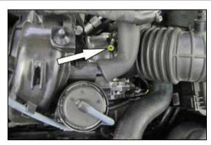
4. Loosen the hose clamp securing the factory intake hose to the throttle body.
