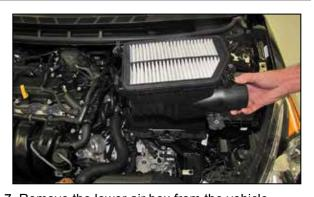
7. Remove the lower air box from the vehicle. NOTE: K&N Engineering, Inc., recommends that customers do not discard factory air intake.
