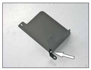
12. Install the heat shield mounting bracket (070015) onto the heat shield and secure with the provided hardware.
