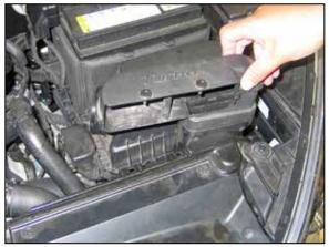
6. Pull the fresh air intake scoop straight up and out of the vehicle.
