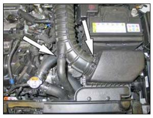
3. Loosen the hose clamp securing the intake hose to the air box and release the spring clamp securing the air injection hose and then disconnect the air injection hose.
