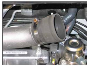
17. Install the provided silicone hose (08096) onto the turbo inlet as shown and secure with the provided hose clamp.
