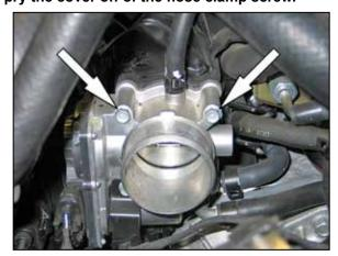
9. Remove the two upper throttle body mounting bolts shown.
