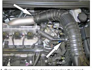
4. Release the spring clamp securing the crank case vent hose and then disconnect the crank case vent hose. Loosen the hose clamp securing the intake hose to the turbo inlet and then disconnect and remove the intake hose from the vehicle.
