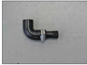
21. Install the provided hose mender into the  $90^{\circ}$  air injection hose and secure with the provided hose clamp.
