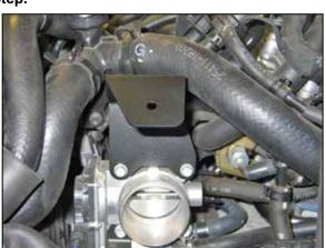
10. Install the provided tube mounting bracket (064303) onto the throttle body and secure with the factory bolts from the previous step.
