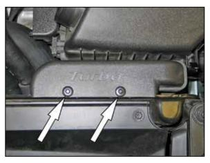
5. Push the centers of the retaining pins down to release the fresh air intake scoop.
