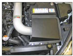
27. Install the cover onto the heat shield and then secure it to the heat shield and core support with the hardware provided.
