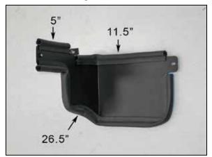
14. Install the three section of edge trim onto the heat shield as shown.
