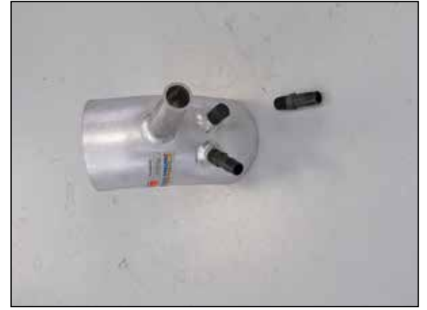
17. Install the provided fittings into the K&N® intake tube as shown.
