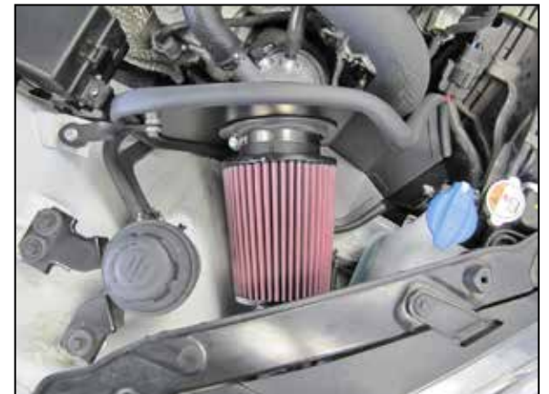
20. Install the K&N® air filter and secure with the provided hose clamp.
