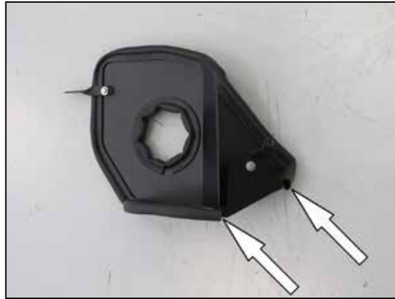
13. Install the 46" section of edge trim around the outside of the heat shield as shown.
