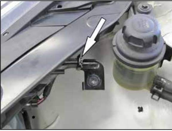
7. Remove the factory air box mounting bracket shown from the back of the headlight.
