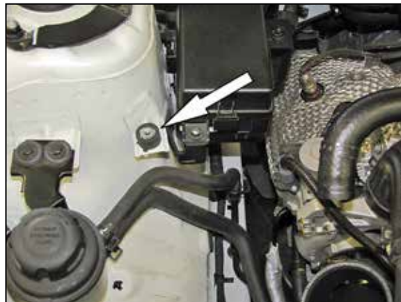
14. Install the provided rubber mounted stud onto the factory air box mounting location on the inner fender.
