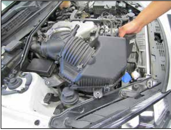
7. Lift up and remove the air box from the vehicle. NOTE: K&N Engineering, Inc., recommends that customers do not discard factory air intake.
