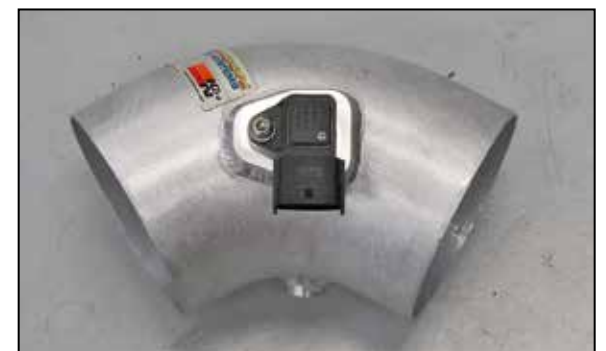
22. Install the air sensor into the K&N® intake tube and secure with the provided hardware.
