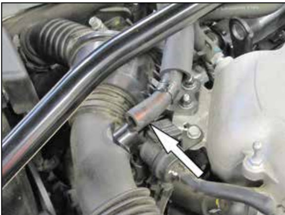
9. Disconnect the vent line from the engine sound tube. NOTE: Some vehicles may not be equipped with a vent line attached to the sound tube.
