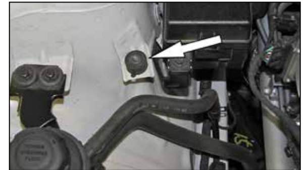
18. Install the provided rubber mounted stud onto the air box mounting location on the inner fender as shown.
