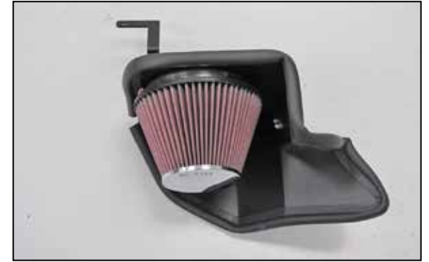
17. Install the K&N® air filter onto the filter adapter and secure with the provided hose clamp.
