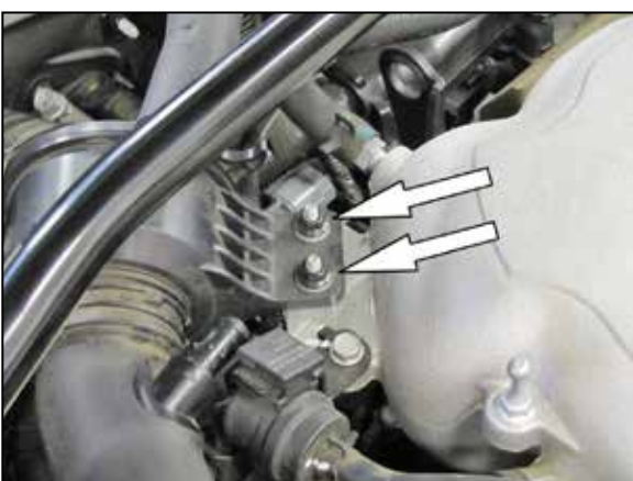
10. Remove the two nuts securing the engine sound drum to the intake manifold.
