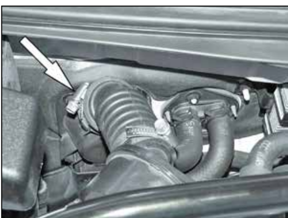
11. Loosen the hose clamp securing the engine sound tube to the fitting in the firewall.
