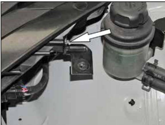
8. Remove the air box mounting bracket from the back of the headlight.
