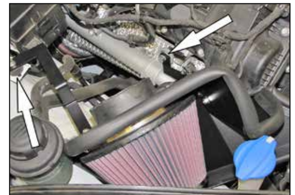
20. Set the filter assembly into position and secure to the rubber mount and coolant tube mounting location with the provided hardware. NOTE: Be sure to place the spacer between bracket #064305 and the coolant tube bracket.
