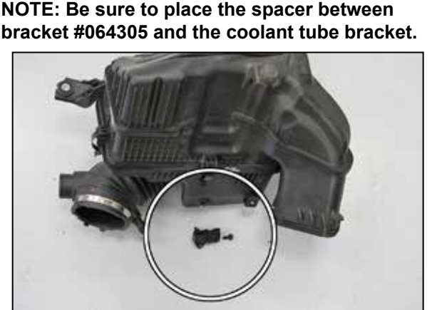
21. Remove the bolt securing the air sensor into the factory air box and then remove the sensor.
