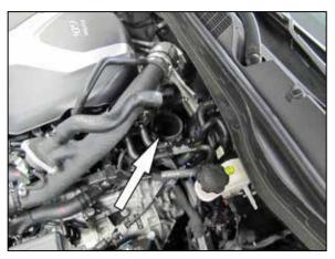
7. Install the provided 90° elbow hose (08504) onto the turbo inlet and secure with the provided hose clamp.
