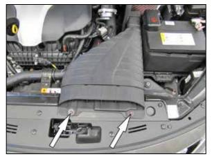
21. Reinstall the fresh air intake scoop and secure with the factory hardware.
