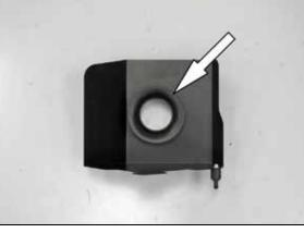
13. Install the air filter adapter into the heat shield and secure with the provided hardware.
