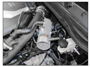
9. Set the K&N<sup>®</sup> intake tube into position in the silicone hose; do not completely tighten the hose clamp at this time.
