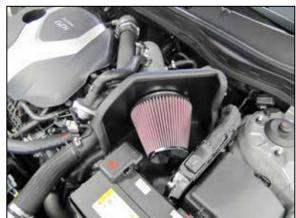
20. Install the K&N<sup>®</sup> air filter and secure with the provided hose clamp.
