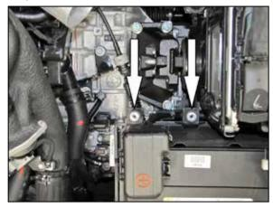
10. Install the two  $\frac{1}{2}$ " high rubber mounted studs provided into the air box mount bolt locations.
