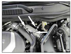
19. Connect the Blow of valve hose, EVAP hose and crank case vent hose to the intake tube and secure with the provided hose clamps.
