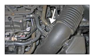
4. On vehicles equipped with EVAP vent line, release the spring clamp and then disconnect the EVAP vent line from the factory intake tube.
