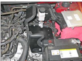
18. Install the heat shield assembly into position and secure to the previously installed rubber mounted studs using the provided hardware.
