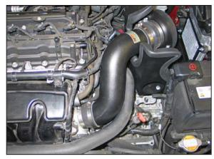
27. Install the K&N® intake tube into the silicone hose at the filter adapter and then into the hose at the throttle body and then secure with the provided hose clamp.
