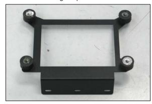
19. Install four rubber mounted studs to the ECU mounting bracket and secure with the provided hardware.
