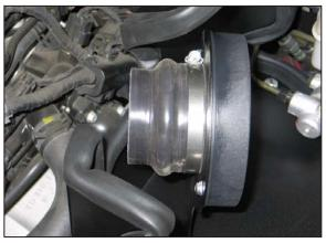
25. Install the provided hump hose (084079) onto the filter adapter and secure with the provided hose clamp.
