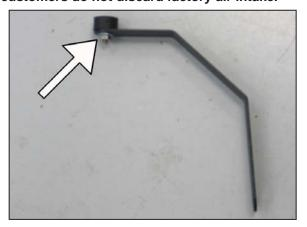
11. Install the ½" rubber mounted stud onto the heat shield mounting bracket (083159) as shown.
