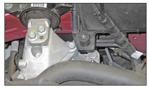
16. Attach the provided 1.0" rubber mounted stud to the battery tray as shown.
