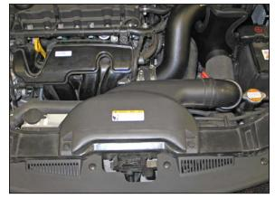
31. Reinstall the fresh air intake scoop onto the core support and secure with the factory mounting bolts. Insert the fresh air intake tube into the hole in the heat shield.
