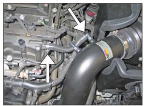
29.Install the provided silicone hose onto the 90° fitting installed into the K&N® intake tube and then attach the open end to the valve cover port and secure with the provided hose clamp.
