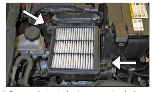
8. Remove the two bolts shown securing the lower airbox.
