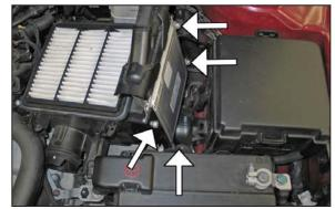
9. Lift the airbox/ECU assembly up and lean it towards the engine, then remove the four bolts securing the ECU to the airbox.
