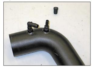
26. Install the two vent fittings into the  $K\&N^{\mbox{\scriptsize @}}$  intake tube as shown.
