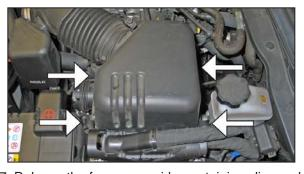
7. Release the four upper airbox retaining clips and then remove the upper airbox and intake tube from the vehicle.
