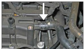
3. Release the spring clamp and then disconnect the crankcase vent hose from the valve cover port.
