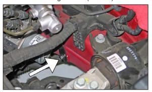
12. Remove the specified bolt securing the ABS pump bracket to the inner fender.
