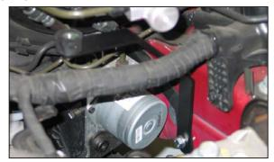
13. Install the heat shield mounting bracket assembly using the provided hardware.
