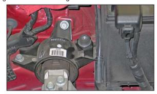
15. Using the provided fender washers, secure the  $\frac{1}{2}$ " rubber mounted stud to the airbox mounting bracket as shown.
