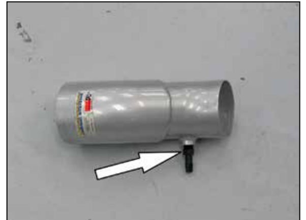
19. Install the provided vent fitting into the K&N® intake tube as shown. NOTE: Plastic NPT fittings are easy to cross thread. Install the vent fitting "hand" tight, then turn it two complete turns with a wrench.
