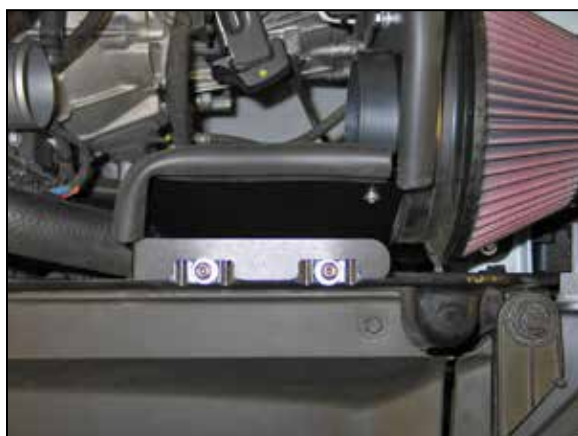
16. Install the fresh air intake scoop and secure to the core support and heat shield/filter adapter with the provided hardware.
