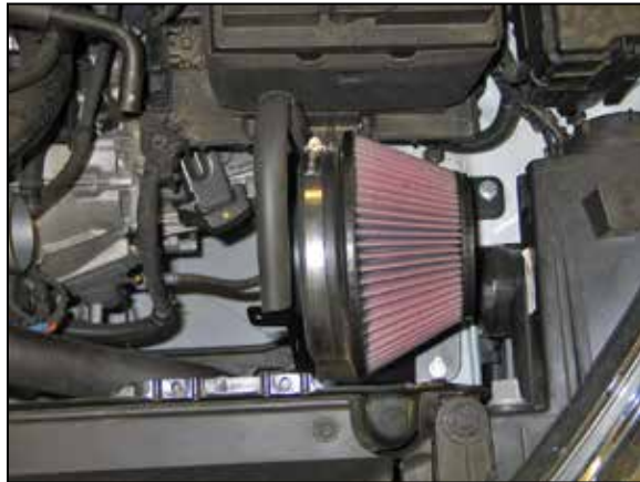
15. Install the filter assembly into the heat shield and secure with the rear mounting bolt provided only at this time. NOTE: Precharger® air filter wrap; part # 22-8036PK is available to purchase separately.
