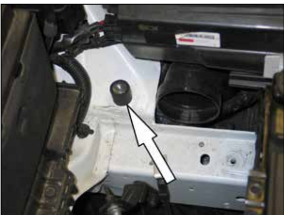
11. Install the 1" rubber mounted stud into the rear factory air box mounting location as shown.
