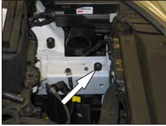
12. Install the 1/2" rubber mounted stud into the front factory air box mounting location as shown.
