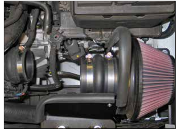
18. Install the provided silicone hump hose (5-576) onto the filter adapter and secure with the provided hose clamp.
