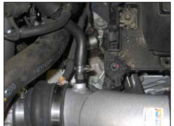
21. Reroute the crank case vent line under the fuel line and then install it onto the crank case vent fitting on the intake tube. Secure with the provided hose clamp.
