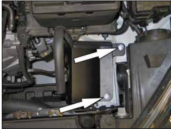
13. Set the heat shield into position on the rubber mounted studs and secure with the provided hardware.
