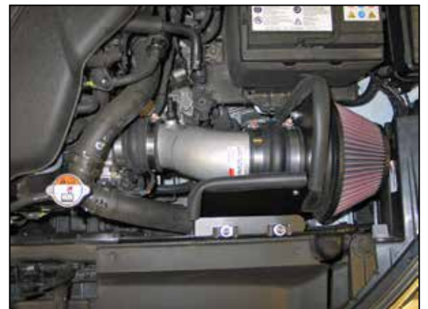
20. Install the K&N® intake tube into the silicone hose at the throttle body fully then into the silicone hose at the filter adapter, adjust the tube for proper fit and then secure with the provided hose clamps.
