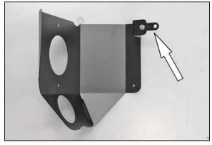
13a. On 2013 and later model vehicles, install the provided bracket (07133) onto the heat shield as shown,
