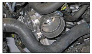
17. Install the provided silicone hose (084036) onto the throttle body and secure with the provided hose clamp.
