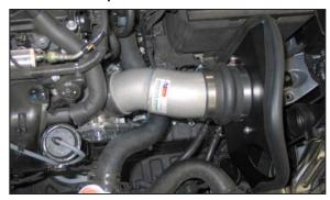
20. Install the K&N<sup>®</sup> intake tube into the silicone hump hose and then into the silicone hose attached to the throttle body. Secure with the provided hardware.
