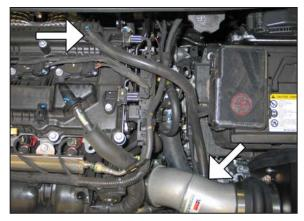
23. Install the provided crank case vent hose onto the 90° fitting in the K&N $^{\odot}$  intake tube. Attach the opposite end to the valve cover vent port.
