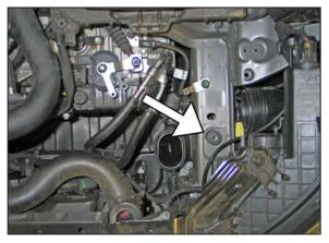
12. Install the 1" rubber mounted stud as shown into the front air box mounting location.
