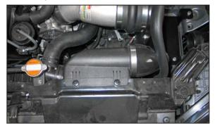
22. Install the fresh air intake scoop assembly so the silicone hose passes through the hole in the heat shield, then secure with the factory retaining clips.
