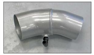
19. Install the provided 90° vent fitting into the K&N® intake tube as shown. NOTE: Plastic NPT fittings are easy to cross thread. Install the vent fitting "hand" tight, then turn it two complete turns with a wrench.
