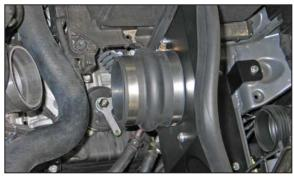
18. Install the provided hump hose (5-576) onto the filter adapter and secure with the provided hose clamp.
