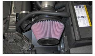
24. Install the K&N<sup>®</sup> air filter and secure with the provided hose clamp.
