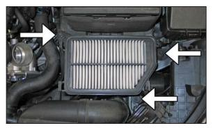
7. Remove the three bolts that secure the lower air box vehicle.
