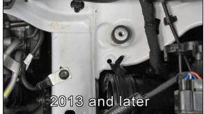
13. Install the  $\frac{1}{2}$ " rubber mounted stud into the rear/inner air box mounting box location. NOTE: On 2011 and 2012 model year vehicles, the rubber mounted stud will go into the inner most threaded hole. On 2013 and later vehicles this position was eliminated and the rubber mounted stud is to be installed in the remaining position.
