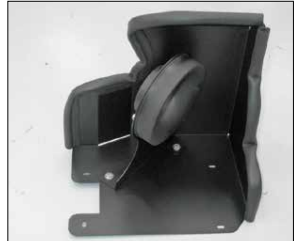
20. Install the bracket assembly onto the heat shield as shown using the provided hardware. NOTE: Do not completely tighten at this time.
