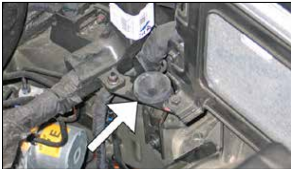
10. Remove the airbox mounting grommet shown.
