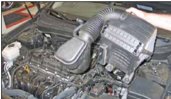
9. Remove the airbox assembly from the vehicle. NOTE: K&N Engineering, Inc., recommends that customers do not discard factory air intake.
