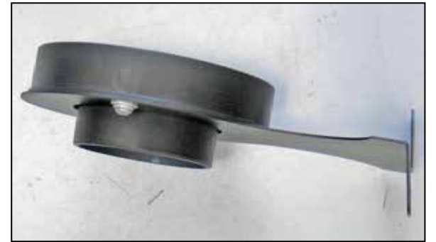
19. Install the filter adapter onto the mounting bracket as shown using the provided hardware. NOTE: The radius adapter will cover over the bracket part number when properly installed.
