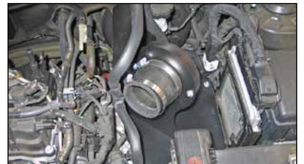
22. Install the provided silicone hose (08724) onto the filter adapter and secure with the provided hose clamps.
