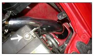
35. Reconnect the negative battery cable and double check that everything is tight and properly positioned before starting the vehicle.
