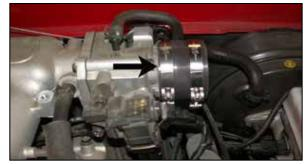
17. Install the silicone hose and hose clamps onto the throttle body and secure as shown.
