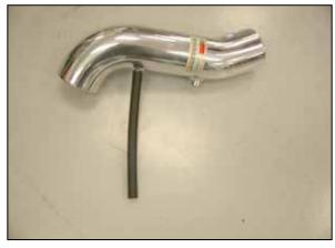
20. Install the provided hose onto the K&N $^{\! @}$  intake tube as shown.
