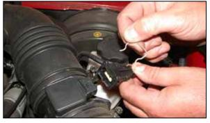
5. Remove the wire clip, then, disconnect the mass air sensor electrical connection as shown.
