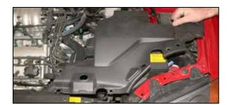
10. Remove the battery cover, which is secured by 4 plastic rivets and one bolt as shown.
