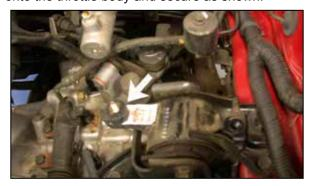
18. Install the provided rubber mounted stud into the original air cleaner mounting hole as shown.
