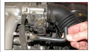
6. Disconnect the crank case vent hose and remove from the engine as shown.
