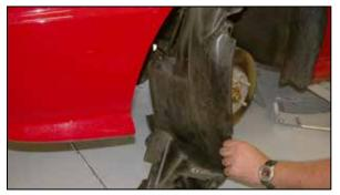
12. Remove five plastic rivets and one bolt, then, pull in the inner fender valance down as shown.
