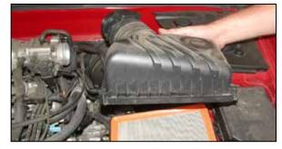
8. Unclip the air cleaner cover and remove as shown.
