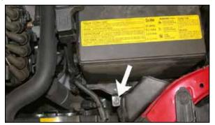
13. Remove the bolt that secures the air inlet duct to the battery tray as shown.
