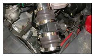
25. Slide the mass air sensor assembly onto the throttle body tube and snug the hose clamp but do not tighten completely at this time.
