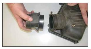
23. Remove the mass air sensor from the air cleaner cover as shown.
