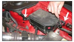
31. Secure the fuse box using the original bolts.
