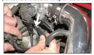
22. Connect the crank case vent hose to the crank case vent as shown.
