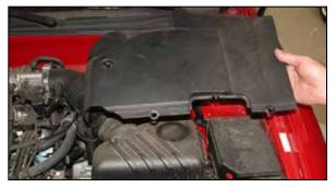
4. Remove the two plastic rivets and one bolt, then, remove the air cleaner cover as shown.
