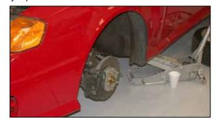
11. Raise the vehicle up and support it with a jack stand, then, remove the front tire as shown.
