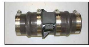
24. Install the two silicone hump hoses and hose clamps onto the mass air sensor and secure as shown.
