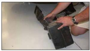
15. From underneath the vehicle remove the two bolts and one clip, then, remove the resonator from the vehicle as shown.
