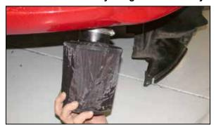
30. Install the K&N $^{\odot}$  air filter from under the vehicle and secure with the provided hose clamp as shown
