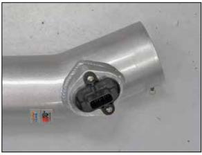
15. Install the mass air sensor into the K&N<sup>®</sup> intake tube and secure with the provided hardware.
