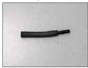
18. Install the provided quick disconnect union into the provided crank case breather hose.
