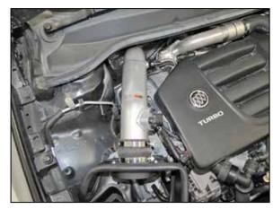
17. Install the K&N® intake tube into the turbo coupler and then into the filter adapter coupler. Adjust the tube and heat shield for best fit and then secure the hose clamps and heat shield hardware.
