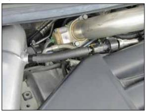
19. Install the crank case breather assembly into the factory quick disconnect fitting and then onto the vent fitting installed into the K&N® intake tube. NOTE: Some trimming of the vent hose may be necessary.
