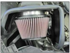
21. Install the K&N® air filter and secure with the provided hose clamp.
