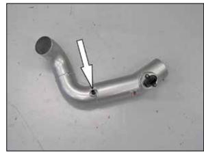
16. Install the provided vent fitting into the  $K\&N^{\otimes}$  intake tube as shown.
