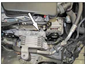
11. Remove the front motor mount bolt shown.
