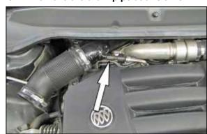
6. Disconnect the crank case vent quick disconnect fitting and then loosen the hose clamp that secures the intake tube to the turbo inlet. Remove the intake hose assembly.
