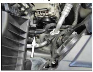
4. Disconnect the air filter housing drain.
