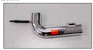
20. Install the EVAP hose assembly onto the K&N $^{\circ}$  intake tube as shown.
