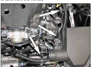
6. Release the three flexible clamps that secure the sound tube and disconnect the sound drum from the rear sound tube then remove the sound tube
