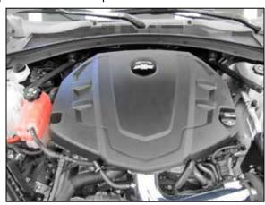
29. Reinstall the decorative engine cover and secure with the factory bolt and oil cap.
