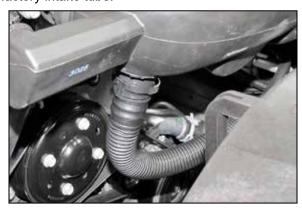
4. Release the sound tube quick disconnect fitting and disconnect the sound tube from the factory intake tube.
