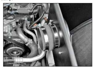
18. Install the provided hump coupler (084079) onto the filter adapter and secure with the provided hose clamp.
