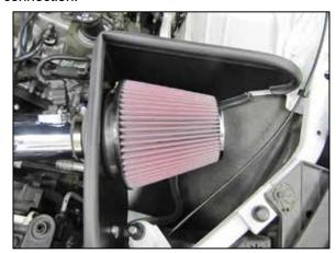
28. Install the  $K\&N^{\odot}$  air filter and secure with the provided hose clamp.
