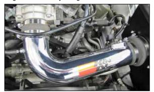
26. Install the provided crank case vent hose onto the factory vent hose and K&N $^{\!0}$  fitting.
