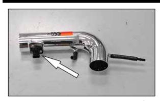
23. Install the mass air assembly into the K&N<sup>®</sup> intake tube as shown.
