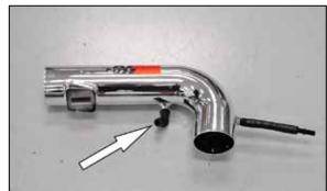
21. Install the 90\* crank case vent fitting into the K&N intake tube as shown.
