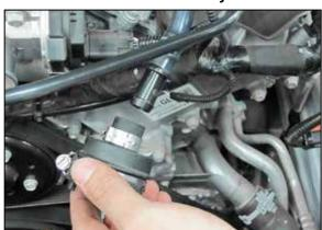
11. Remove the factory crank case vent coupler from the crank case vent tube.
