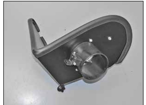
19. Install the mass air sensor into the K&N® mass air housing and secure with the provided hardware.
