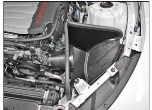
20. Install the K&N® heat shield assembly onto the air filter housing mounting grommets.
