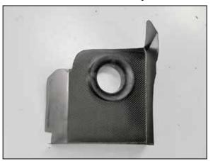
8. <u>Install the provided air filter adapter</u> into the K&N<sup>®</sup> heat shield and secure with the provided hardware.
