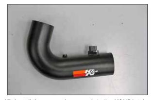
17. Install the mass air sensor into the K&N $^{\! \otimes}$  intake tube and secure with the provided hardware.
