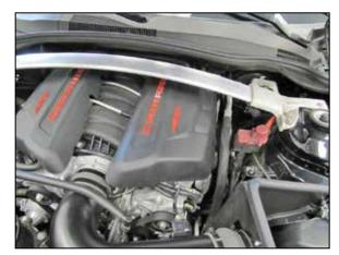
22. Reinstall the driver's side engine cover.
