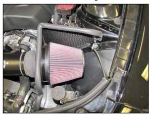
23. Install the K&N $^{\odot}$  air filter and secure with the provided hose clamp.
