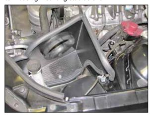
13. Install the heat shield assembly into the vehicle so that the mounting bracket slides onto the mounting stud and the mounting stud inserts into the factory mounting bracket. Then secure the heat shield with the factory nut and secure the ground strap to the threaded stud with the factory fastener.
