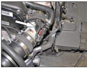
19. Connect the Pressure sensor to the quick disconnect fitting installed into the K&N® intake tube.
