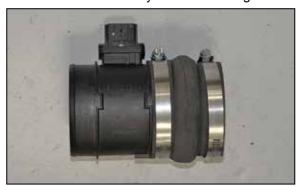
16. Install the provided hump coupler (087121) onto the mass air sensor as shown and secure with the provided hose clamp.
