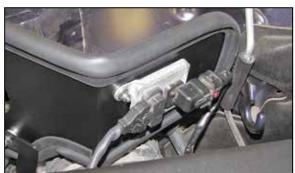
10. Using the provided hardware, secure the electrical box to the heat shield as shown.
