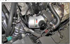
14. Install the K&N® intake tube into the coupler at the turbo but do completely tighten at this time.
