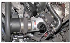
17. Slip the mass air sensor through the hole in the heat shield and then slide the coupler hose onto the K&N® intake tube. Adjust the tube and hoses for best fit and then secure the hose clamps.
