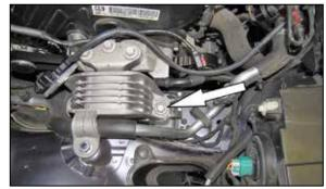
6. Remove the motor mount bolt show.
