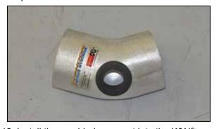
12. Install the provided grommet into the K&N® intake tube as shown.
