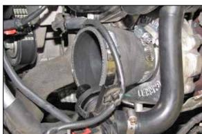
11. Install the provided step coupler (08713) onto the turbo inlet and secure with the provided hose clamp.
