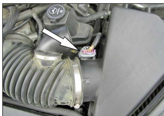
4. Disconnect the mass air sensor electrical connection.
