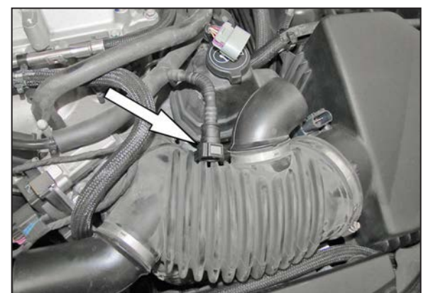
5. Disconnect the crank case vent line from the factory quick disconnect fitting.
