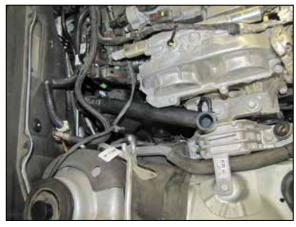
13. On vehicles equipped with air injection, Install the provided air injection hose (08479) onto the factory union and secure with provided hose clamp. **NOTE: Do not completely tighten at this time.**
