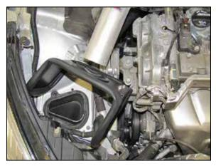
27. Set the heat shield onto the engine mount so the bracket lines up with the engine mounting bolt hole. Reinstall the engine mounting bolt.
