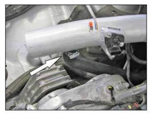
22. On vehicles equipped with air injection, connect the hose to the fitting in the intake tube and secure with the provided hose clamp.
