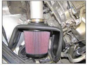
28. Install the K&N<sup>®</sup> air filter and secure with the provided hose clamp.
