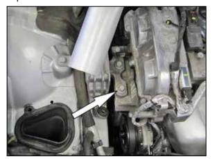
26. Remove the front engine mounting bolt shown.
