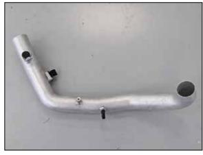
18. Install the provided npt vent fitting into the  $K\&N^{\circledast}$  intake tube as shown.
