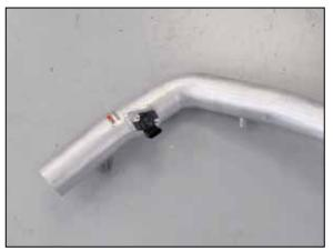
16. Install the mass air sensor into the  $K\&N^{\otimes}$  intake tube as shown.
