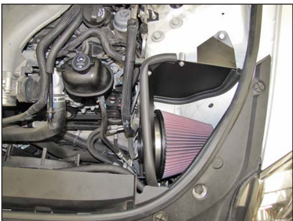
17. Install the heat shield and filter assembly into the engine compartment and secure it the fan shroud with the factory bolt and to the inner fender with the hardware provided. NOTE: be sure to place the provided rubber fender washer between the heat shield and inner fender. Due to manufacturer tolerances, the transmission coolant tube may need to be adjusted to prevent contact with the heat shield mounting bracket.
