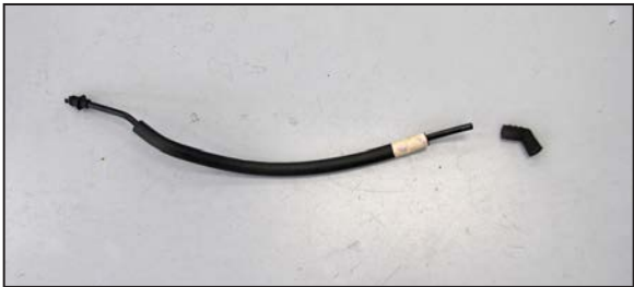
18. Remove the crank case vent tube from the valve cover and then remove the factory elbow from the tube as shown.
