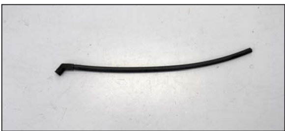
20. Attach the provided crank case vent hose to the hose mender as shown and then reattach the factory elbow to the valve cover.
