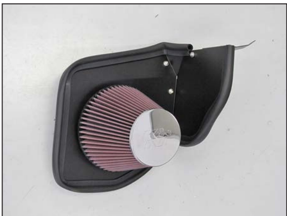
15. Install the K&N® air filter onto the filter adapter and secure with the provided hose clamp. NOTE: Drycharger® air filter wrap; part # RC-5107DKDK is available to purchase separately.
