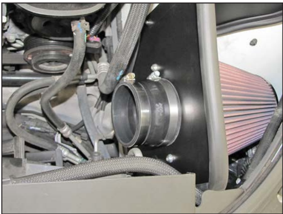
21. Install the provided hose (08051) onto the filter adapter and secure with the provided hose clamp.
