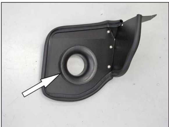
12. Install the filter adapter into the heat shield as shown using the provided hardware.
