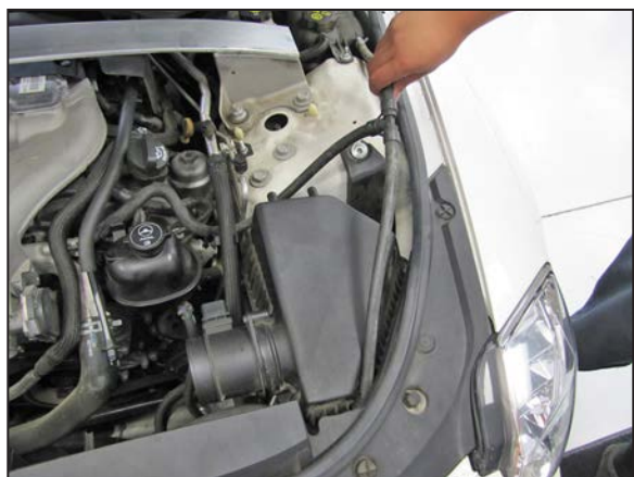
8. Unhook the coolant by-pass hoses and lift them up and over the air filter housing.
