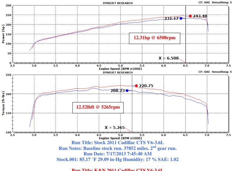
Run Title: K&N 2011 Cadillac CTS V6-3.6L Run Notes: K&N intake kit #69-4528 installed. 37582 miles. 2<sup>nd</sup> gear run. Run Date: 7/17/2013 9:01:14 AM K&N.002: 83.32 °F 29.06 in-Hg Humidity: 18 % SAE: 1.02
