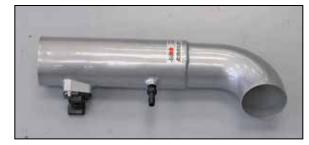
21. Install the provided crank case vent into the  $K\&N^{\otimes}$  intake tube as shown.
