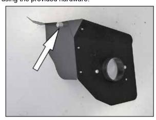
11. Install the provided aluminum stand-off onto the heat shield as shown using the provided hardware.
