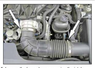
5. Loosen the hose clamps securing the intake tube to the throttle body and air filter housing, then remove the intake tube and crank case vent from the vehicle.
