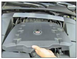
2. Remove the oil fill cap and then lift off the engine cover. Reinstall the oil cap after the engine cover has been removed.
