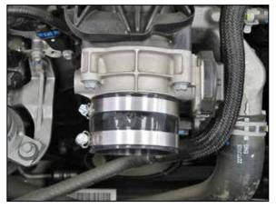
17. Install the provided hose (08434) onto the throttle body and secure with the provided hose clamps.
