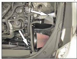
16. Set the heat shield assembly into position and secure it the fan shroud and inner fender with the factory bolts.
