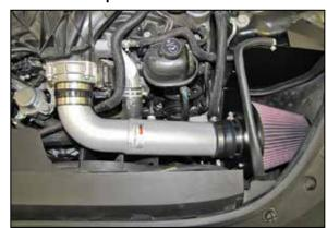
22. Install the K&N® intake tube into the hose at the filter adapter and then into the hose on the throttle body, align the tube for proper fit and then secure with the provided hose clamps.
