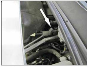
4. Disconnect the crank case vent tube coupler from the rear of the driver's side valve cover.
