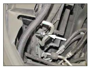
15. Remove the fan shroud mounting bolt shown. **NOTE: This bolt will be reused in the next step.**
