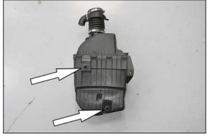
8. Remove two of the factory mounting grommets from the air box.
