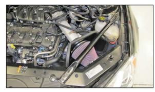
30. Reinstall the body brace and secure with the factory hardware.
