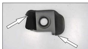
16. Install the provided edge trim onto the heat shield as shown.
