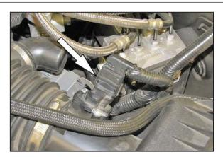
4. Release the red locking tab and then disconnect the mass air sensor electrical connection.
