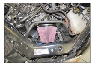
21. Install the heat shield assembly into the vehicle so the mounting grommets set onto the mounting studs.
