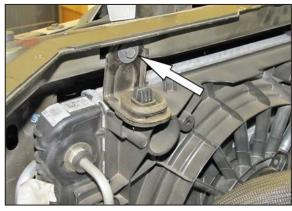
19. Remove the bolt shown that secures the radiator mount to the core support.
