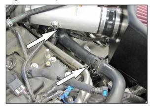
27. On vehicles equipped with air injection, install the air injection hose onto the K&N<sup>®</sup> intake tube and then connect it with the factory air injection tube.
