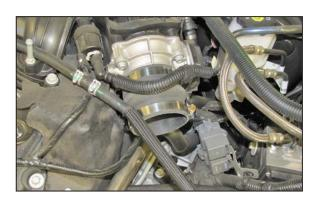
18. Install the provided hump hose (08696) onto the throttle body and secure with the provided hose clamp.
