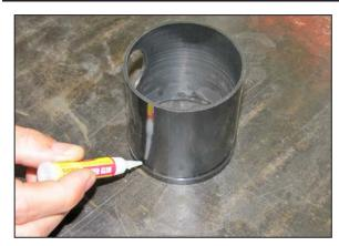
10. Apply several drops of the provided glue to the mass air insert as shown.
