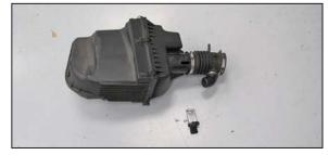
9. Remove the two screws securing the mass air sensor and then remove the sensor from the air box.
