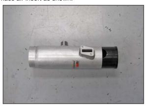
11. Install the mass air insert into the K&N<sup>®</sup> intake tube so that the hole in the insert aligns with the mass air location in the tube.
