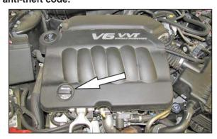
2. Remove the oil fill cap and then remove the engine cover from the engine. Reinstall the oil fill cap.
