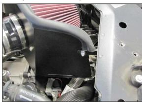
24. Secure the heat shield to the mounting bracket with the hardware provided.
