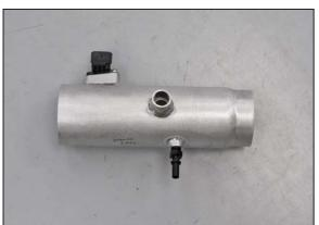
13. Install the provided NPT quick disconnect fitting into the  $K\&N^{\otimes}$  intake tube as shown.
