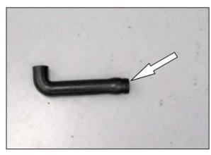
26. On vehicles equipped with air injection, install the provided quick disconnect fitting in to the straight end of the provided hose.
