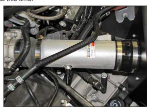
23. Install the K&N® intake tube into the hose at the throttle body and align the tube with the filter adapter. Slide the hose into position and secure with the provided hose clamps.
