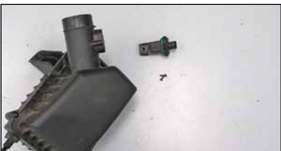
11. Remove the two screws securing the mass air sensor into the factory air box and then remove the mass air sensor from the air.
