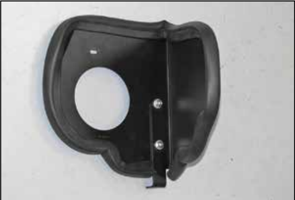
8. Install the provided edge trim onto the heat shield as shown. NOTE: Some trimming of the edge trim will be necessary.
