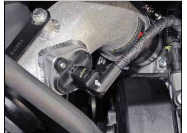
18. Reconnect the mass air sensor electrical connection.
