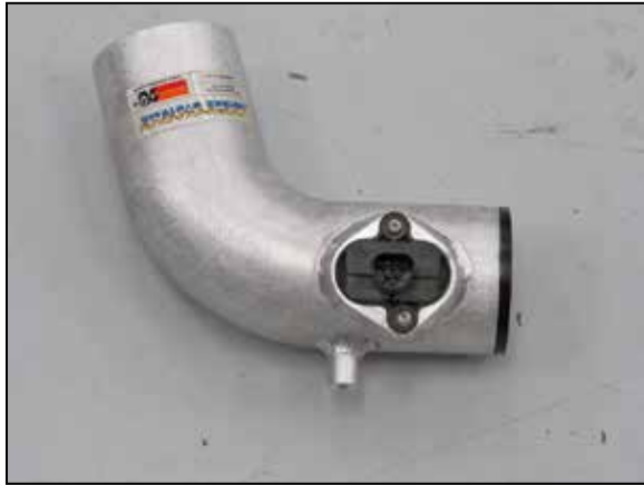
12. Install the mass air sensor into the K&N® intake tube and secure with the provided hardware.
