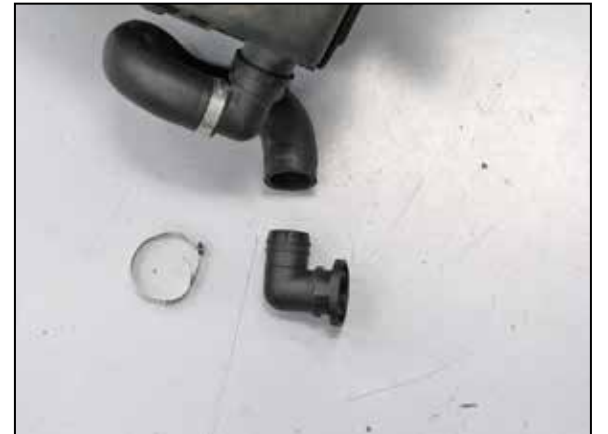
18a. On vehicles equipped with air injection, release the clamp securing the factory air injection fitting to the hose and then remove the fitting from the hose.
