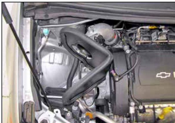
15. Set the Heat shield assembly along with the provided spacer onto the engine mount and secure with the engine mounting bolt removed in step #13.
