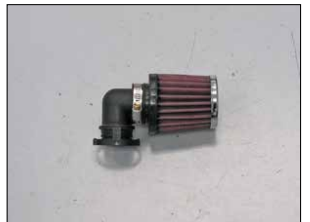
18b. On vehicles equipped with air injection, install the provided breather filter onto the factory fitting from step #11a as shown and secure with the provided hose clamp.
