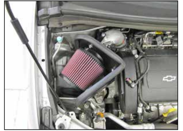
17. Install the K&N® air filter onto the intake tube and secure with the provided hose clamp. NOTE: Drycharger® air filter wrap; part # RX-4990DK is available to purchase separately.
