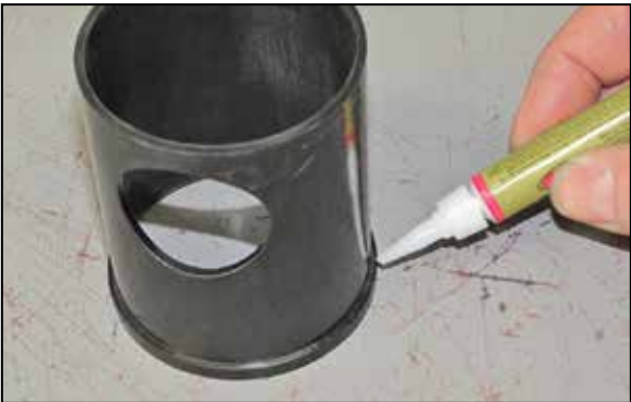
9. Apply several drops of the provided "Super Glue" to the lip of the venturi as shown.
