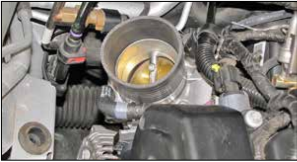
6. Install the silicone hose (084016) onto the throttle body and secure with the provided hose clamp.
