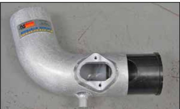
10. Install the venturi into the K&N® intake tube so that the hole lines up with the mass air sensor adapter. NOTE: Some tapping may be needed to fully seat the venturi into the intake tube.
