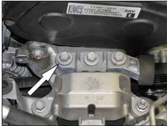
13. Remove the rear engine mounting bolt shown. NOTE: This bolt will be reused.
