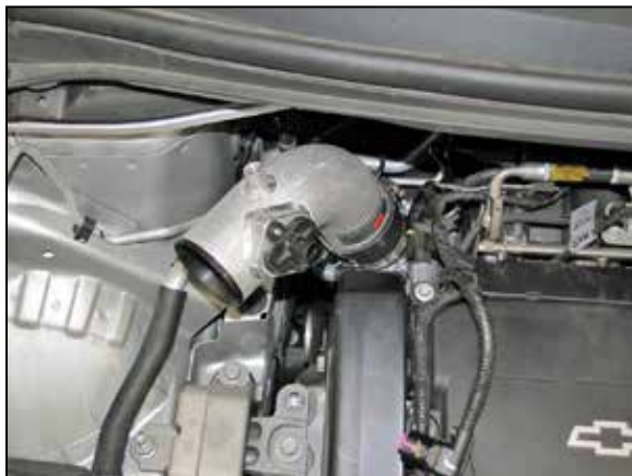
14. Install the K&N® intake tube into the silicone hose but do not completely tighten at this time.
