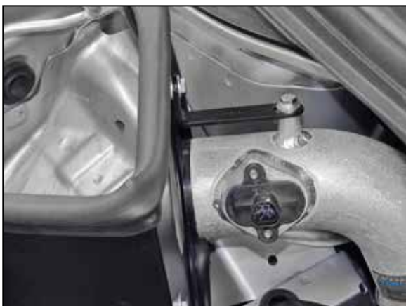
16. Install the tube mounting bracket (010051) onto the heat shield along with the provided spacer. Align the tube and heat shield for proper fit and then secure the bracket, heat shield and intake tube with the provided hardware.
