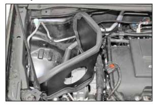
8. Install the heat shield assembly onto the engine mount and secure with the bolt removed in step #5. **NOTE: Do not completely tighten at this time.**
