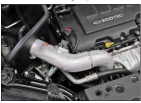
17. Install the tube assembly into the silicone hose on the turbo inlet and align so the rubber mounted stud protrudes through the heat shield. Secure the tube with hose clamp and hardware provided.
