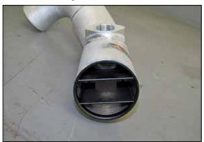
12. Install the air guide into the  $K\&N^{\otimes}$  intake tube as shown.
