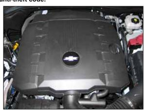
2. Remove the oil fill cap and then lift up and remove the engine cover. Reinstall the oil cap.
