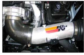
20. Remove the 90° vent hose from the crank case vent tube. Then install the provided silicone vent hose; trim the hose for proper fit and install it onto the fitting installed into the K&N® intake tube.
