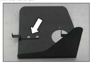
9. Install the heat shield mounting bracket (083126) onto the heat shield and secure with the provided hardware.
