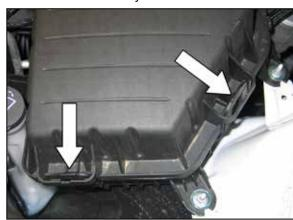
6. Unlatch the upper air box clips and then remove the upper air box and intake tube assembly.
