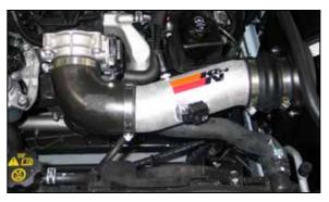
19. Install the provided silicone hose (08629) onto the K&N® intake tube as shown. Install the K&N® intake tube assembly onto the throttle body and filter adapter, adjust the tube in the hoses for proper fitment. Once properly fitted, secure the tube with the provided hose clamps.
