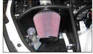
21. Install the K&N® air filter and secure with the provided hose clamp.
