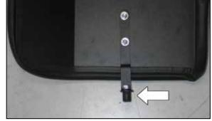
12. Install the provided inserted nut onto the heat shield mounting bracket and secure with the provided hardware.
