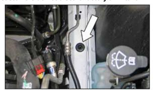
8. Remove the air box mounting grommet shown from the frame rail.
