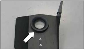
10. Install the filter adapter into the heat shield and secure with the provided hardware.
