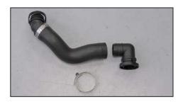
22. On vehicles equipped with air injection, remove the air injection hose from the factory air box. Cut the band clamp and disconnect the 90° quick disconnect fitting from the air injection hose.
