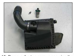
15. Remove the two screws securing the mass air sensor into the factory air box; remove the sensor from the air box.
