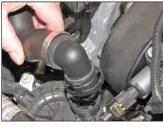
5. On vehicles equipped with "Air Injection". Disconnect the air injection hose from the air injection pump as shown.
