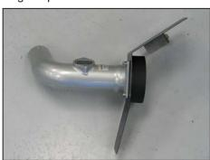
14. Install the filter adapter and K&N<sup>®</sup> intake tube onto the heat shield as shown using the provided hardware and gaskets.
