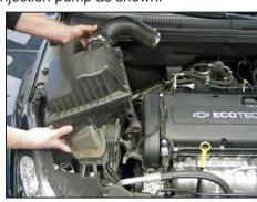
6. Lift up the air box assembly to dislodge it from the mounting grommets; then remove the air box assembly from the vehicle.
