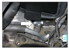
19. Secure the intake assembly with the provided hardware and hose clamp.
