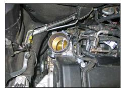
8. Install the provided silicone hose (084014) onto the throttle body and secure with the provided hose clamp.
