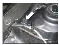
10. Remove the plastic plug and then install the inserted nut into the strut tower as shown.
