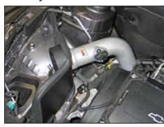
18. Set the intake assembly into position so the intake tube is inserted into the silicone hose, the rubber insert mounts into the front lower air box mount and the rubber mounted stud is attached to the heat shield.
