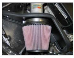
20. Install the K&N® air filter onto the filter adapter and secure with the provided hose clamp.
