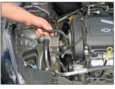
7. Remove the air box drain pipe from the vehicle. NOTE: The drain pipe is connected to the inner fender by two plastic clips that will need to be removed or clipped.
