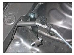
11. Install the heat shield bracket assembly onto the strut tower as shown using the provided hardware.
