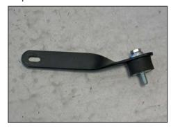
9. Install the provided rubber mounted stud onto the provided heat shield bracket (07945) as shown.
