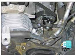
9. Install the heat shield mounting bracket onto the motor mount and secure with the factory bolt removed in step #7.
