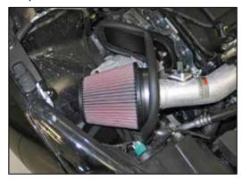
17. Install the  $K\&N^{\otimes}$  air filter onto the filter adapter and secure with the provided hose clamp.
