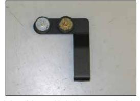
8. Install the provided rubber mounted studs onto the heat shield mounting bracket as shown.
