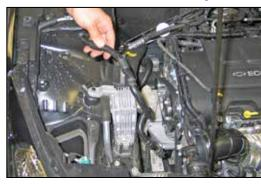
6. Unhook the two clips that secure the airbox drain tube to the inner fender, and then remove the drain tube from the vehicle.
