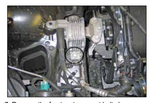
7. Remove the front motor mount bolt shown. **NOTE: This bolt will be reused in a later step.**
