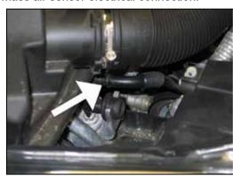
3. Disconnect the airbox drain tube from the airbox. **NOTE:** The drain tube will pull straight out from the airbox.
