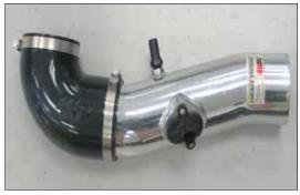
19. Install the provide elbow hose (08629) onto the K&N intake tube as shown and secure with the provided hose clamp.
