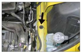
8. Remove the air box mounting grommet shown from the inner fender.
