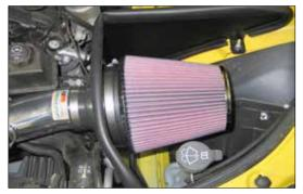
22. Install the K&N air filter and secure with the provided hose clamp. NOTE: Drycharger<sup>®</sup> air filter wrap; part #
