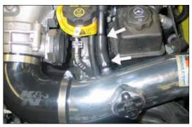
21. Install the provided silicone hose onto the factory crank case vent tube and then connect the open end onto the vent fitting installed into the K&N intake tube.
