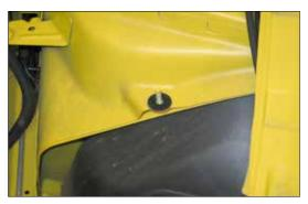
13. Install the provided rubber fender washer onto the outward air box mounting stud.
