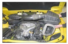
7. Remove the factory air box assembly from the vehicle.
