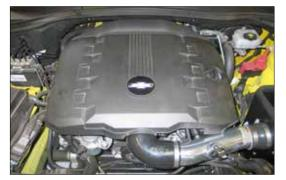
24. Reinstall the engine cover and secure with the oil fill cap.
