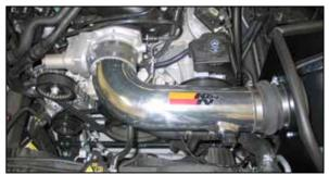
21. Install the K&N<sup>®</sup> intake tube assembly into the silicone hose at the filter adapter and then into the silicone hose at the throttle body and secure with the provided hose clamps.
