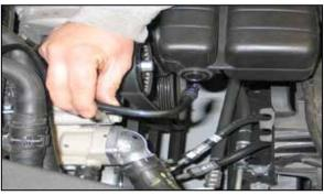
4. Disconnect the crank case vent tube from the intake resonator as shown.
