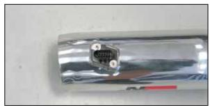
19. Install the mass air sensor into the  $K\&N^{\otimes}$  intake tube and secure with the provided hardware.
