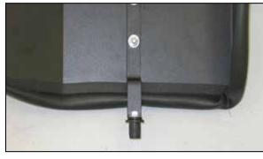
14. Install the inserted nut onto the heat shield mounting bracket using the provided hardware. Do not completely tighten at this time.
