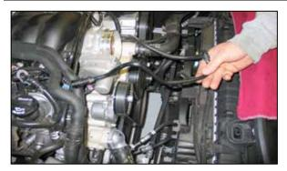
7. Rotate the crank case vent tube 180°, then release the retainer at the valve cover port and the remove the crank case vent tube.
