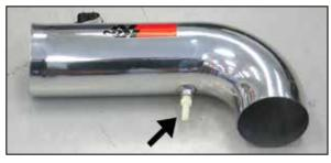
20. Install the provided 1/4npt fitting into the  $K\&N^{\circledast}$  intake tube as shown.
