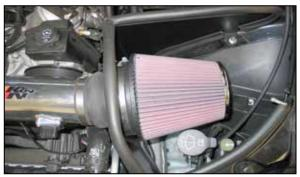
23. Install the K&N<sup>®</sup> air filter onto the filter adapter and secure with the provided hose clamp. **NOTE: Drycharger<sup>®</sup> air filter wrap; part # RF-1042DK is available to purchase separately.**
