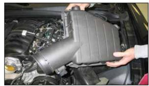
9. Lift up and remove the air box from the vehicle. NOTE: K&N Engineering, Inc., recommends that customers do not discard factory air intake.
