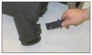
18. Remove the two screws and then remove the mass air sensor from the factory air box.
