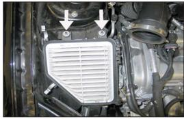
5. Remove the two lower air box retaining nuts shown.
