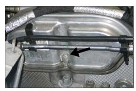
9a. On vehicles not equipped with a valve cover mounted engine id plate, lift the bypass hose assembly up from the mounting boss then remove the valve cover bolt shown.
