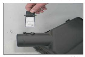
13. Remove the two mass air sensor retaining screws and then remove the mass air sensor from the air box as shown.
