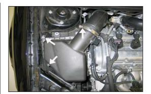
4. Loosen the hose clamp which secures the intake tube to the air box, release the two retaining clips and then remove the air box lid from the vehicle.
