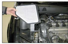
6. Pull up the lower air box to release it from the mounting gourmet and then remove the lower air box from the vehicle.
