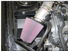
22. Install the  $K\&N^{\circ}$  air filter and secure with the provided hose clamp.
