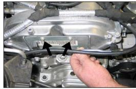
9. Lift the bypass hose assembly up to release it from mounting boss and then on vehicles equipped with an engine id plate, remove the two bolts shown.
