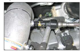
21. Connect the crank case vent hose to the quick connect fitting on the  $K\&N^{\rm @}$  intake tube.
