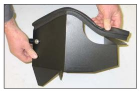
18. Install the provided edge trim onto the heat shield. Some trimming of the edge trim will be necessary.
