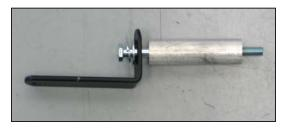
9b. On vehicles not equipped with a valve cover mounting engine id plate, assemble intake tube bracket (070060) using the provided hardware as shown.
