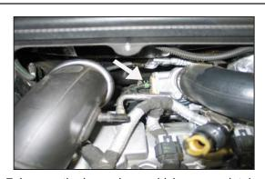
7. Loosen the hose clamp which secures intake tube to the turbo inlet.
