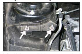
11. Install the two provided spacers onto the air box mounting studs as shown.
