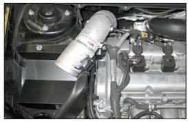
20. Install the K&N® intake tube into position on the turbo inlet and align with the tube mounting bracket. Secure the intake tube with the provided hose clamp and hardware.
