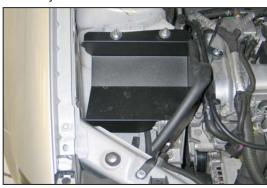
19. Set the heat shield into position on the air box mounting studs. Secure the mounting bracket to the core support with the provided hardware. Secure the heat shield to the mounting studs with the factory nuts removed in step #5.
