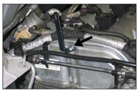
10a. On vehicles not equipped with a valve cover mounted engine id plate, install the tube mounting bracket assembly onto the engine and secure it with the provided hardware. Reinstall the bypass hose assembly back into the mounting boss.
