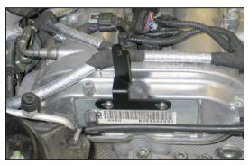
10.On vehicles equipped with a valve cover mounting engine id plate, install the tube mounting bracket (083123) onto the engine and secure it with the provided hardware. Reinstall the bypass hose back into the mounting boss.
