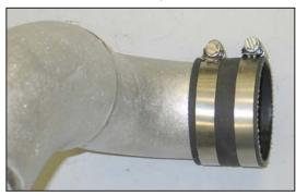
15. Install the provided silicone hose (08727) onto the K&N $^{\odot}$  intake tube and secure with the provided hose clamp.
