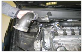
8. Remove the intake tube from the vehicle. NOTE: K&N Engineering, Inc., recommends that customers do not discard factory air intake.
